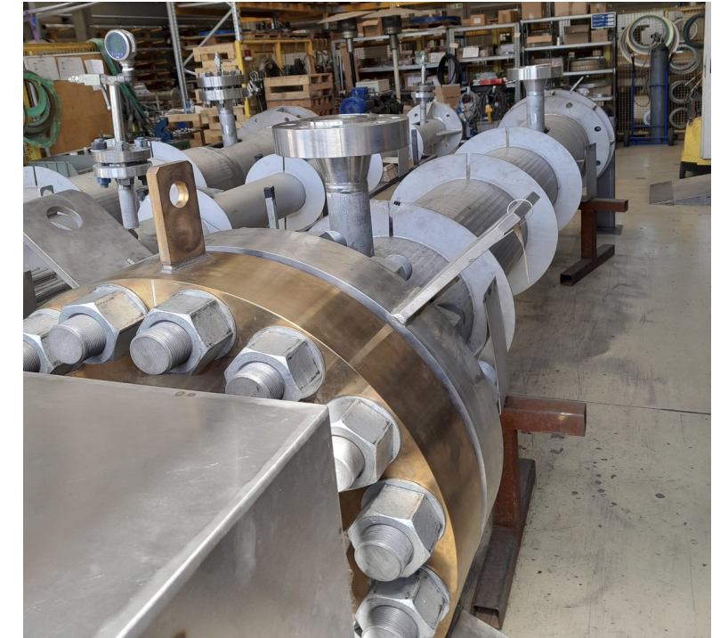
Water Loop 2x1700kW electrical heaters
