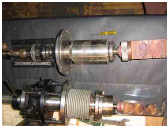
Fig. 3 - Target holders with water cooling.
