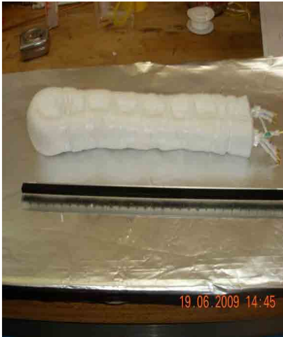
Fig. 1. - Photo of the 3 wires with thermal insulation. Fig. 2. - Photo of the experimental setup.
