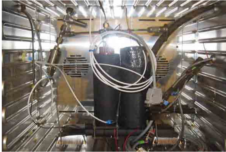
Figure 5. - Fully assembled DTA Calorimeter.
