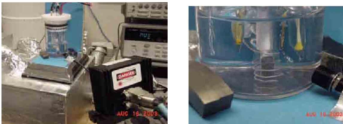
Fig.3. Overall photograph of the excess power experiment and close-up of the electrochemical cell in Texas.
