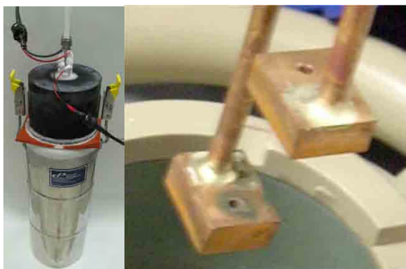
Fig. 2 - Photographs of the cryogenic calorimeter and its cathode connection blocks.
