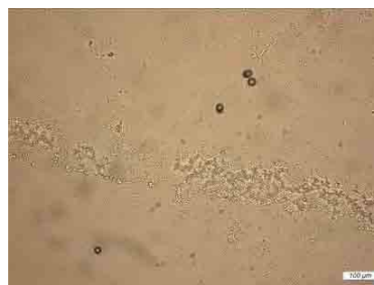
Fig. 9 - Artifacts in CR39 area faced cathode, without Mylar protection
