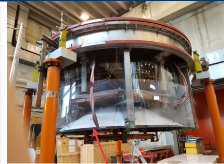
Insulation in Teflon on up & down divertor
