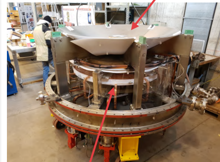
Gas injection also from cathode
