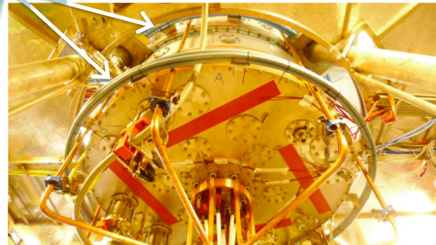
4 additional external PF coils
