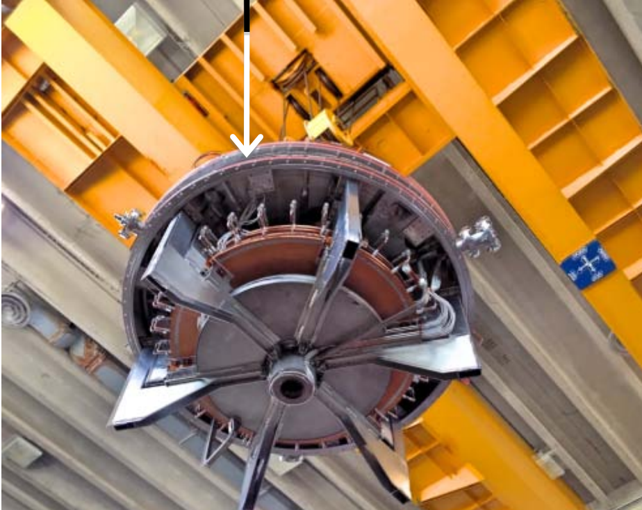
Assembly of the anular anode on the machine (May 2015)
