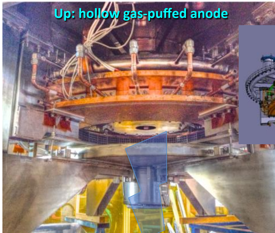
Down: 3000° K heated cathode
