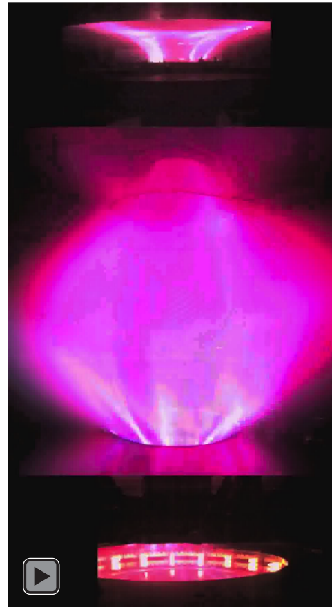
#977, 10 kA Hydrogen break-down V_e \sim 320 V, steady V_e \sim 220 V
