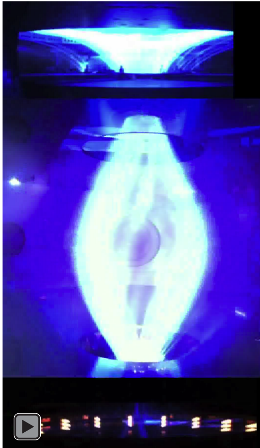
#614, 8.5 kA Argon break-down V_e \sim 90 V, steady V_e \sim 200 V
