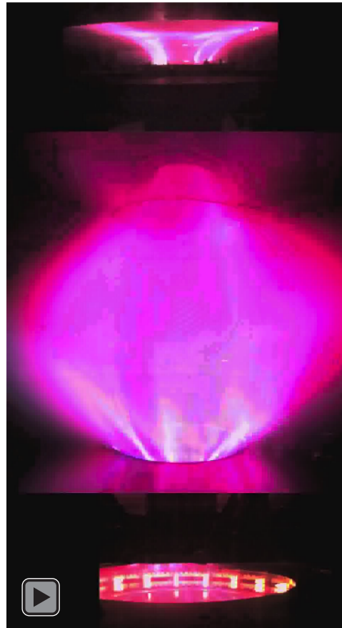
#977, 10 kA Hydrogen break-down V_e \sim 320 V, steady V_e \sim 200 V
