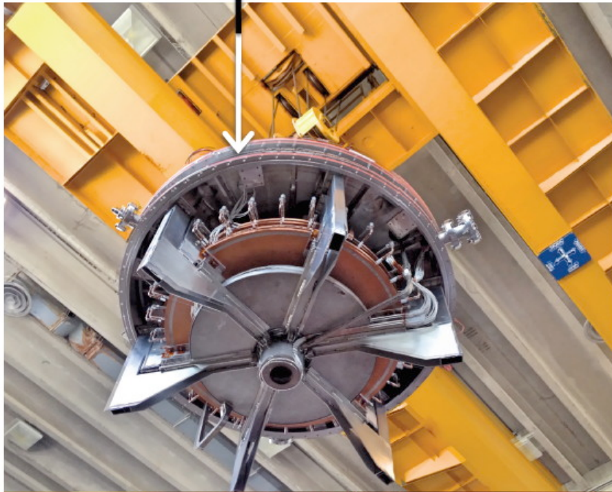
Assembly of the anular anode on the machine (May 2015)
