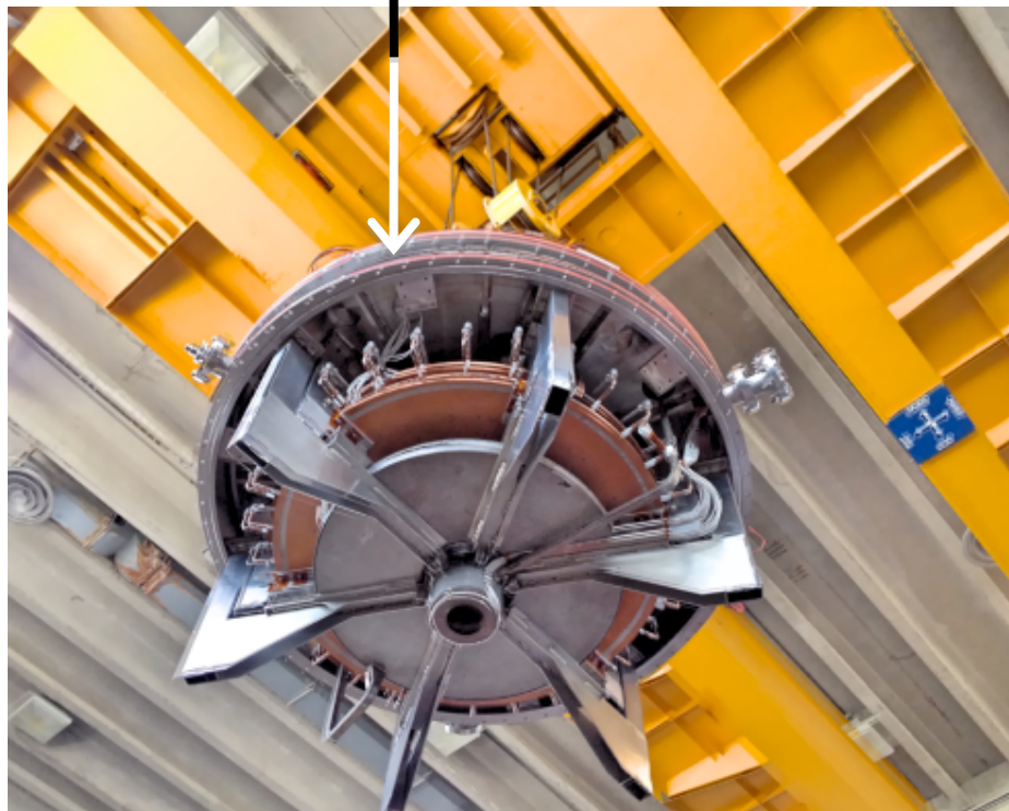
Assembly of the annular anode on the machine (May 2015)
