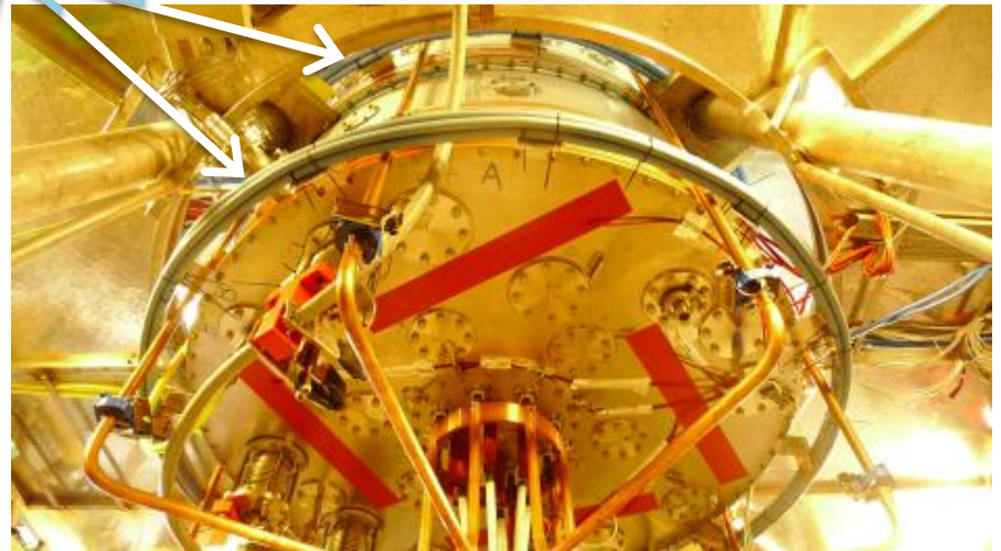
4 additional external PF coils
