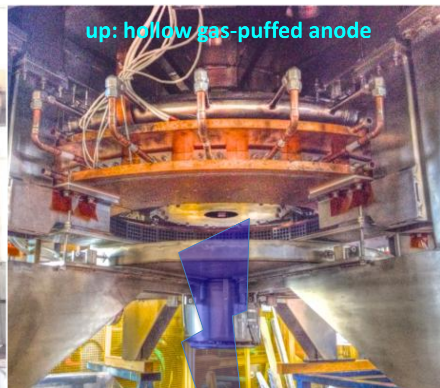
down: 3000° K heated cathode present stage cathode (18 x 3 emitters): aim 10 kA
