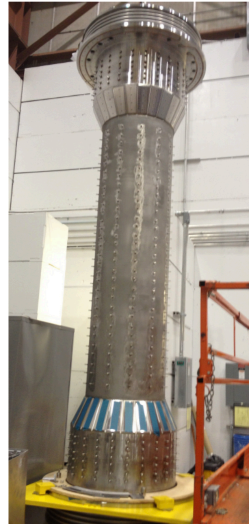
Center-Stack Casing with tile studs
