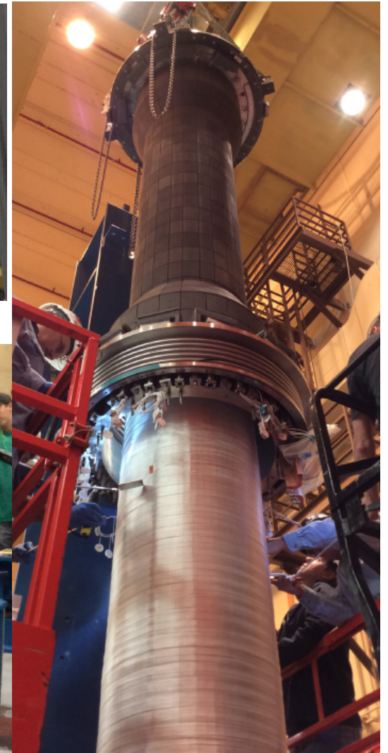
CS Casing lowered onto Center Bundle
