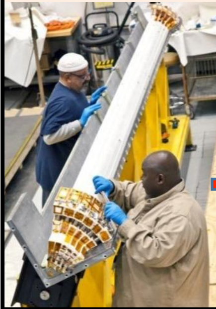
Insulated conductor being placed into mold
