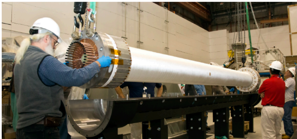
TF bundle with ground wrapping lowered into VPI mold
