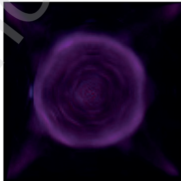
Figure 17: Equatorial cross-section of light emission density of Helium discharge 2154
