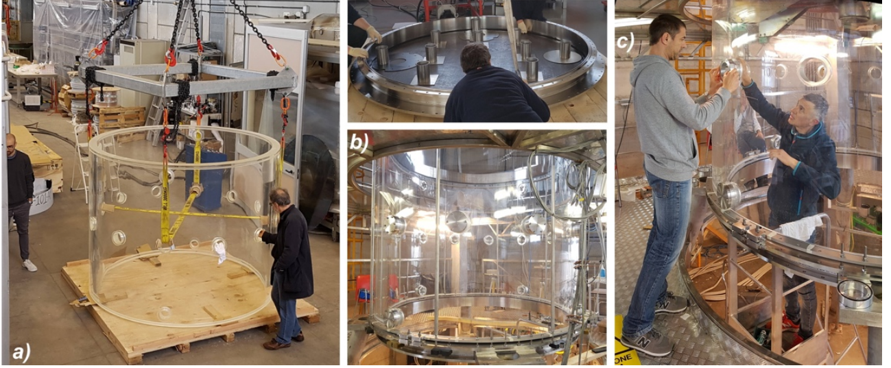
FIGURE 3. (a) The 9 cm thick, 2 m internal diameter, 1.7 m high, new PMMA vessel. (b) One of the two new AISI304 ferrules being tested upon a 10 mm thick Viton flat gasket (top). The new vessel placed in position, with the Viton flat gasket interfacing it with the new bottom ferrule, held by the sustaining legs, pre-charged by compression poles and aligned by brackets (bottom). (c) Closing the diagnostic ports by “bulkhead fitting” technology.
