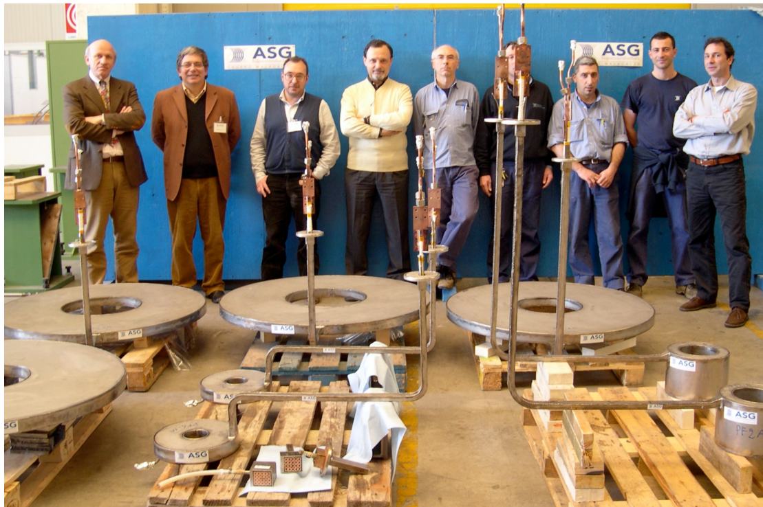
Fig. 5. March 2007: the 4 pairs of MULTI-PINCH PF coils as built by ASG Superconductors.
