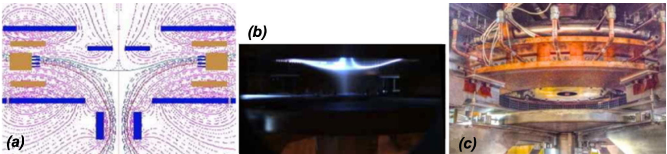
Figure 5. (a) Poloidal cross section map of magnetic lines of force near the anode (yellow), showing the triple X-point on axis, in the middle of the anodic PFInt-B coils (blue). (b) Image of the upper triple X-point, while the plasma centerpost (which lays below) is being switched-off, shot #117. (c) The hollow annular anode.
