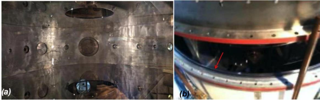
Figure 10. (a) Upper and lower diaphragm glued to the cylindrical large polycarbonate foil with a vacuum compatible strong sealant, able to sustain the diaphragm weight. (b) Polycarbonate insulating spacer ring, vacuum sealed with two o-rings on both sides, inserted between the upper ferrule and the aluminium vessel, sketched also in figure 2(a).
