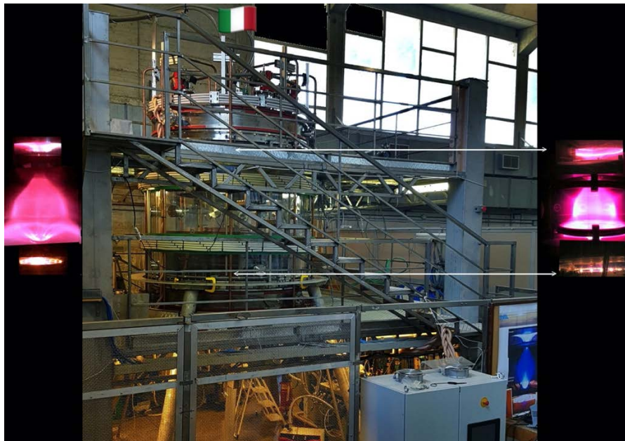
Figure 4: left - first lean torus, obtained in 2018, center – photo of the experiment in 2019, right – fatter hydrogen tori obtained in 2020
