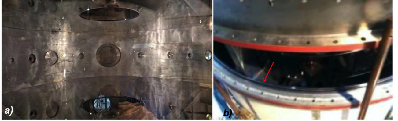
Figure 10. (a) Upper and lower diaphragm glued to the cylindrical large polycarbonate foil with a vacuum compatible strong sealant, able to sustain the diaphragm weight. (b) Polycarbonate insulating spacer ring, vacuum sealed with two o-rings on both sides, inserted between the upper ferrule and the Aluminium vessel, sketched also in Fig. 2(a).
