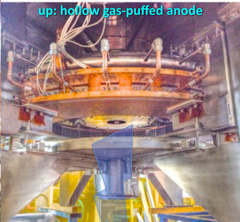
May 2015 annular anode lowered on top of machine
