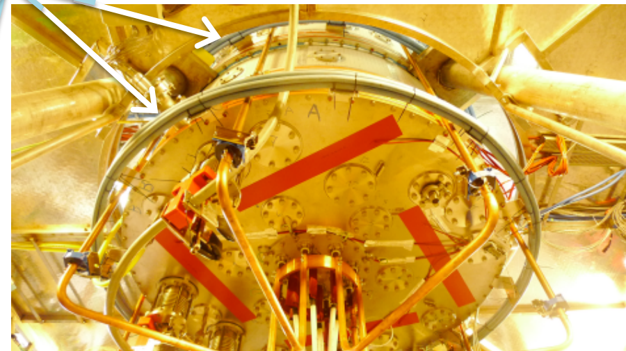
4 additional external PF coils
