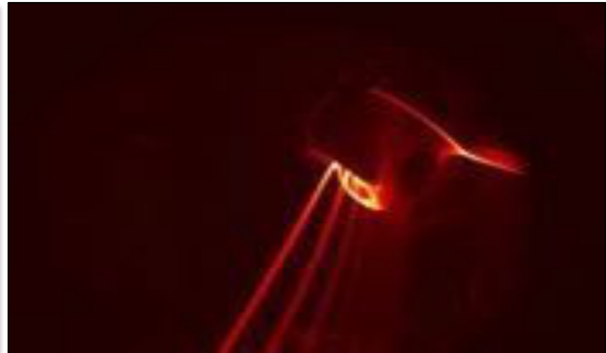
With shear, the e-beam (barely) misses the e-gun on its second toroidal transit
