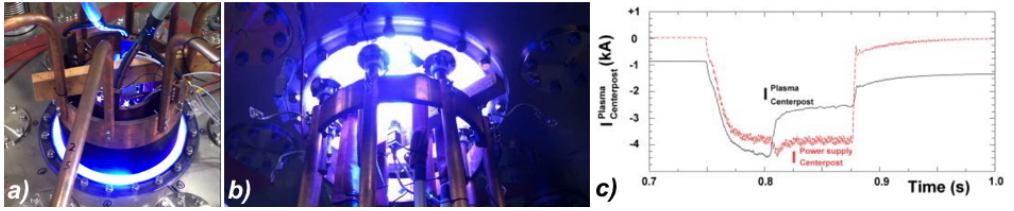
FIGURE 6. (a) The visible light of an Argon plasma centerpost emerging from the upper anodic polycarbonate flange, shot #567. (b) The visible light of an Argon plasma centerpost emerging from the lower cathodic polycarbonate flange, shot #577. (c) Waveforms of Argon centerpost plasma current, evidencing a sudden decrease after the centerpost discharge becomes attached to the Aluminium cylindrical vacuum vessel, shot #208.
