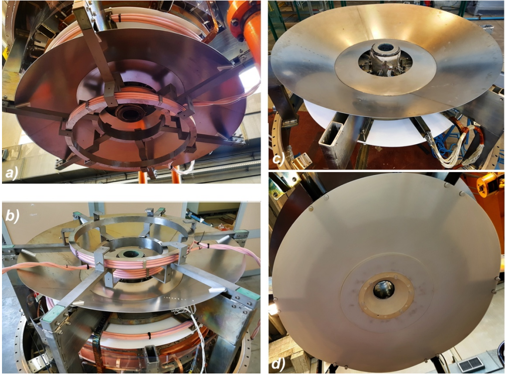
FIGURE 15. The new six PFInt-A compression coils: (a) Two within the upper conical divertor plate and one above it; (b) Two within the lower conical plate and one below it. The green fiberglass blocks insulate the horizontal supports holding the compression coils from the vertical sustaining columns. (c) The new upper conical 2 mm thick AISI304 divertor plate, seen from above; below it the large Teflon diaphragm. (d) The large Teflon diaphragm viewed from below, showing the inner Alumina cone that surrounds the hole inside the lower PF2 mirror coil.
