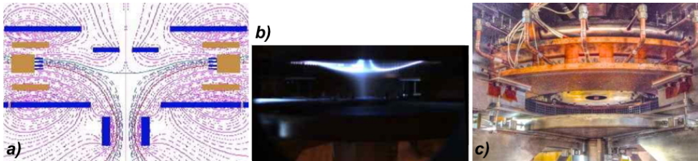
FIGURE 5. (a) Poloidal cross section map of magnetic lines of force near the anode (yellow), showing the triple X-point on axis, in the middle of the anodic PFInt-B coils (blue). (b) Image of the upper triple X-point, while the plasma centerpost (which lays below) is still present but is being switched-off, shot #117. (c) The hollow annular anode.
