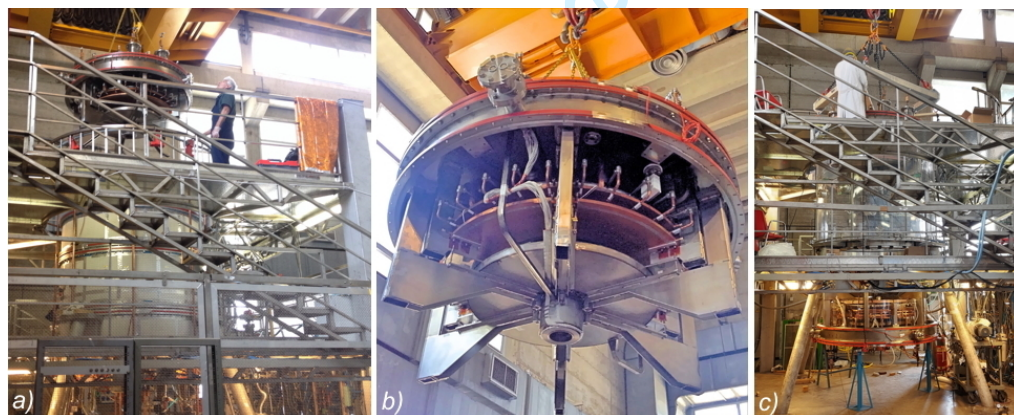
FIGURE 3. (a) The annular anode being lowered on the Aluminium vacuum vessel (2015). (b) Image of the copper anode, on the rear side of which white Teflon blocks and tubes insulate the gas-puffing system from the upper lid; the metal disc below is the PF3.1 coil and the cylinder the PF2 mirror coil, through whose hole the plasma emerges. (c) The annular cathode, below the machine, being lifted into the new PMMA transparent vacuum vessel (since year 2019).
