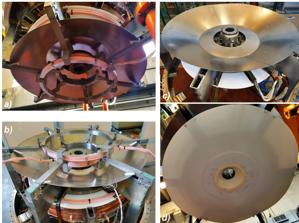
FIGURE 15. The new six PFInt-A compression coils: (a) Two within the upper conical divertor plate and one above it; (b) Two within the lower conical plate and one below it. The green fiberglass blocks insulate the horizontal supports holding the compression coils from the vertical sustaining columns. (c) The new lower conical 2 mm thick AISI304 divertor plate, seen from above; below it the large Teflon diaphragm. (d) The same large Teflon diaphragm seen from below, showing the inner Alumina cone that surrounds the hole inside the lower PF2 mirror coil.
