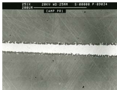
Figure 4 Photomicrograph (250x) of a detail of fig. 3 where diffusion zones of brazing material into base material may be identified
