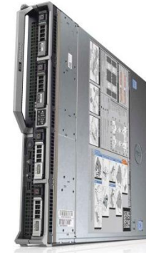
PowerEdge M820 Intel XEON E5-4600 1.5TB RAM (48)
