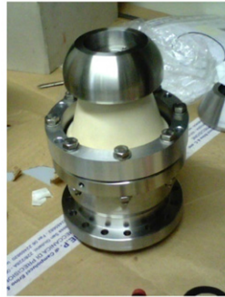
Figure 8. Top: vacuum transmission line and sliding support (actual prototype and conceptual drawing) for a single four-strap antenna; bottom: front-end ceramic feedthrough.
