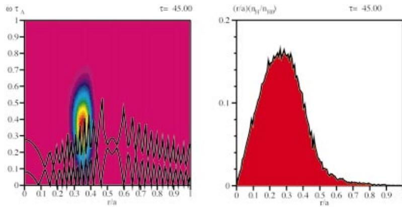
FIG. 11. (Color) Same as Fig. 9, but with a stronger drive. Here,  $\beta_{H0} = 0.022$  and  $t = 45\tau_A$ , in the linear destabilization phase.
