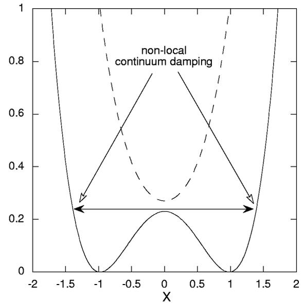
FIG. 3. Radial structure of the shear Alfvén continuous spectrum for the  $(m, n)$  and  $(m-1, n)$  modes in the case  $\Omega_{A,m} + \Omega_{A,m-1} \approx r_0/R_0$ . The value of  $q^2 R_0^2 k_{im,n}^2$  is shown vs  $x \equiv \sqrt{nq_0''}(r-r_0)$ . The frequencies of the even parity toroidal mode is also shown as expected from Eq. (9).
