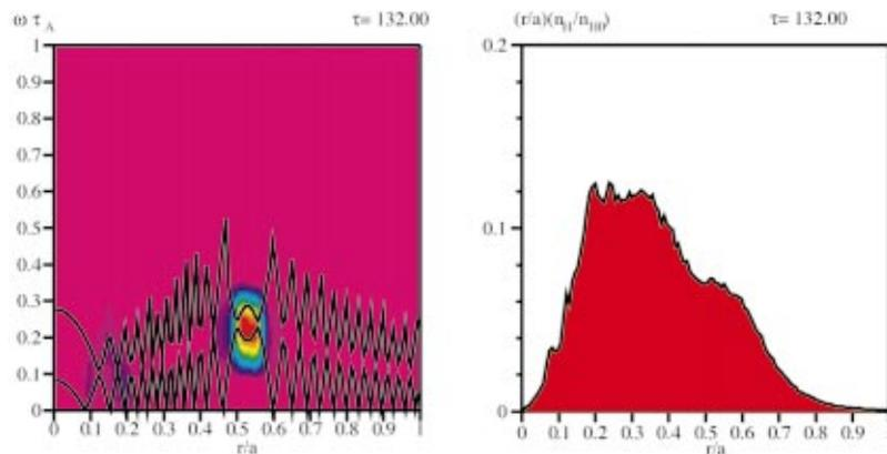
FIG. 12. (Color) Same as Fig. 11, but at  $t = 132\tau_A$ , in the fully nonlinear saturated phase. The fast ion radial distribution (right),  $(r/a)(n_H/n_{H0})$ , shows strong modifications when compared with that of the initial state, confirming significant and rapid radial particle transport.
