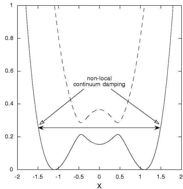
FIG. 4. Radial structure of the shear Alfvén continuous spectrum for the  $(m,n)$  and  $(m-1,n)$  modes for  $\Omega_{A,m} + \Omega_{A,m-1} \ll -r_0/R_0$ . The value of  $q^2 R_0^2 k_{||m,n}^2$  is shown vs  $x \equiv \sqrt{nq_0^n}(r-r_0)$ . The frequencies of the *even parity double EPM* (toroidal mode) is also shown where it could be expected.
