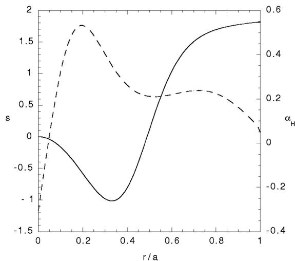
FIG. 6. Radial profile for  $s=rq'/q$  (solid line) and  $\alpha_H$  (broken line).
