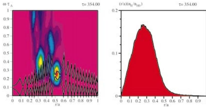
FIG. 10. (Color) Same as Fig. 9, but at  $t = 354\tau_A$ , in the fully nonlinear saturated phase. The fast ion radial distribution (right),  $(r/a)(n_H/n_{H0})$ , does not indicate significant modifications from that of the initial state.
