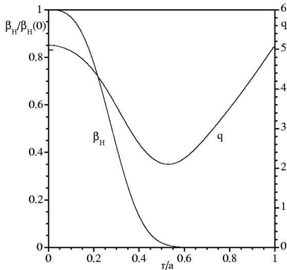
FIG. 8. Radial profiles of  $q$  and  $\beta_H$  that are used in the nonlinear simulations with the HMGC code (Refs. 11 and 12).
