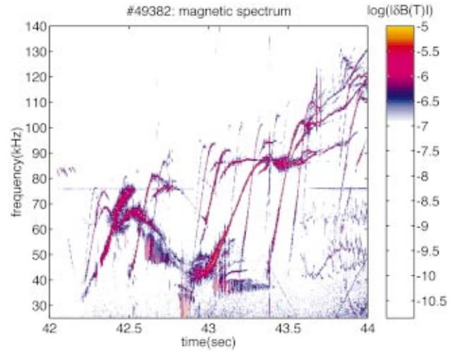
FIG. 2. (Color) Magnetic spectrum in the preheating phase of a JET RS plasma with nonmonotonic  $q$  profile (Ref. 5). See also Ref. 6.
