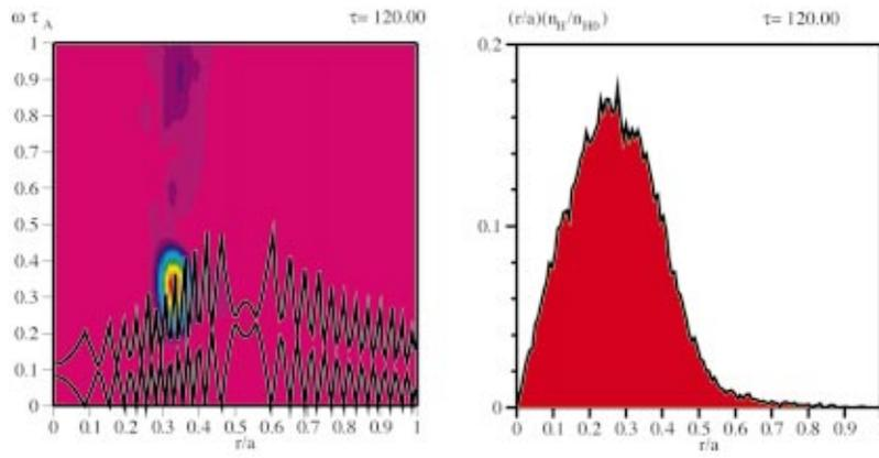
FIG. 9. (Color) Contour plot (left) of the EPM scalar potential fluctuation intensity in the  $(r/a, \omega\tau_A)$  plane at  $\tau = t/\tau_A = 120$ , in the linear destabilization phase. Here,  $\beta_{H0} = 0.008$  and  $\tau_A = R_0/v_A$  is the Alfvén time. The shear Alfvén continuous spectrum is also shown for reference in the background. The initial fast ion radial distribution (right),  $(r/a)(n_H/n_{H0})$ , is also shown as a function of  $r/a$ .
