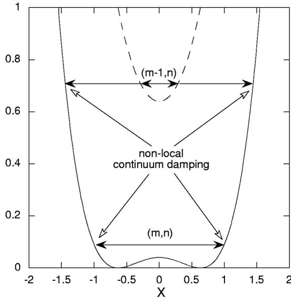
FIG. 1. Radial structure of the shear Alfvén continuous spectrum for the  $(m, n)$  and  $(m-1, n)$  modes in the case  $r_0/R_0 \ll \Omega_{A,m} + \Omega_{A,m-1} \leq 1$ . The value of  $q^2 R_0^2 k_{\parallel m,n}^2$  is shown vs  $x \equiv \sqrt{nq_0''(r-r_0)}$ . The frequencies of the  $(m, n)$  and  $(m-1, n)$  modes are also shown as they are expected from Eq. (3).
