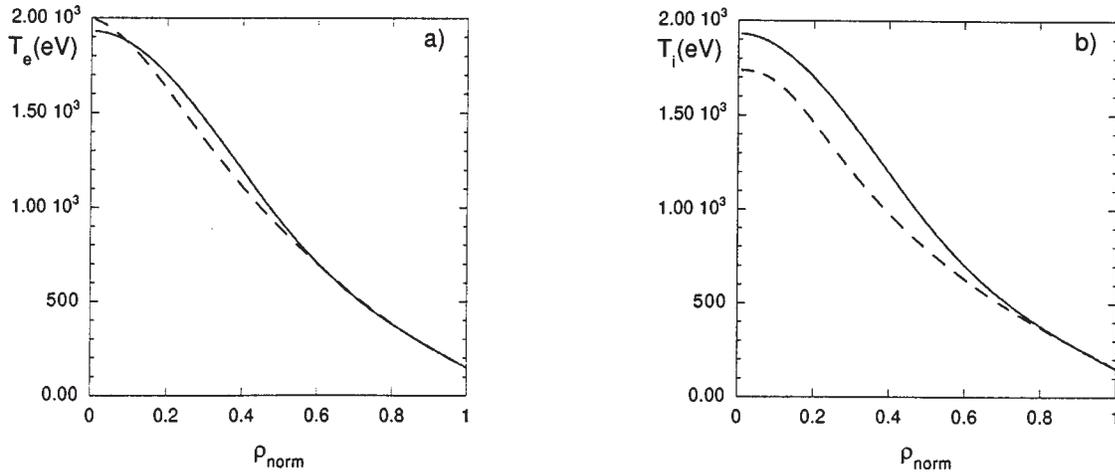
FIG. 3. Experimental (solid curves) and computed (dashed curves) electron (a) and ion (b) temperature profiles for DIII-D discharge 69627 at  $t \simeq 4.4$  s.
