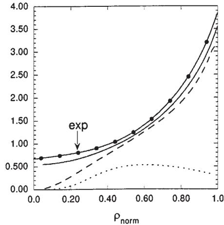
FIG. 4. Safety factor  $q$  (solid curve), shear (dashed curve) and shear dependent function  $f(s)$  (dotted curve) radial profiles for the same discharge as Fig. 3. The safety factor as obtained from the ITER Profile Database is also shown for comparison (solid curve with filled circles labelled ‘exp’).
