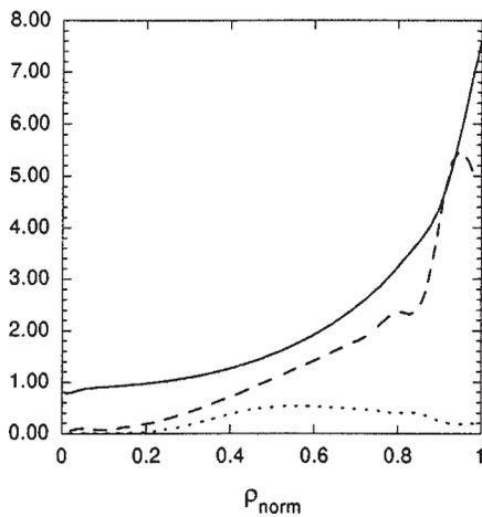
FIG. 14. Safety factor  $q$  (solid curve), shear (dashed curve) and shear dependent function  $f(s)$  (dotted curve) radial profiles for the same discharge as Fig. 13.
