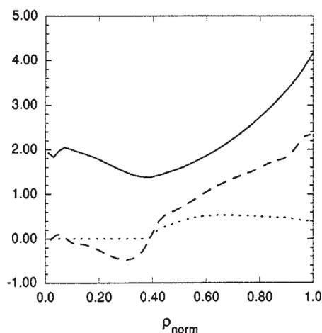
FIG. 11. Safety factor  $q$  (solid curve), shear (dashed curve) and shear dependent function  $f(s)$  (dotted curve) radial profiles for the same discharge as Fig. 10.
