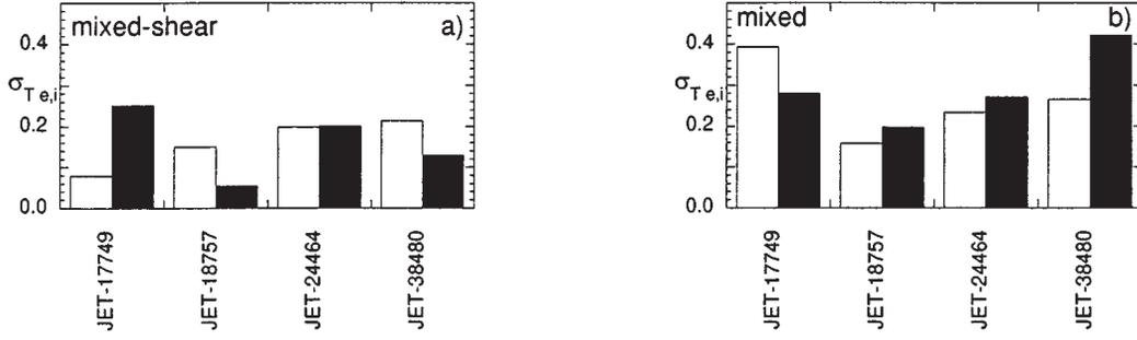
FIG. 8. Electron (white columns) and ion (black columns) temperature standard deviations for the JET hot ion and PEP discharges calculated on the whole cross-section ( $\rho_{\text{norm}} \in [\rho_{\text{norm}}^{\text{min}}, \rho_{\text{norm}}^{\text{max}}] = [0, 1]$ ). The mixed, shear dependent model (a) proposed in this article is compared with the mixed model (b) proposed in Ref. [12].
