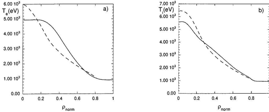
FIG. 2. Experimental (solid curves) and computed (dashed curves) electron (a) and ion (b) temperature profiles for JET discharge 19691 at  $t \simeq 54$  s.
