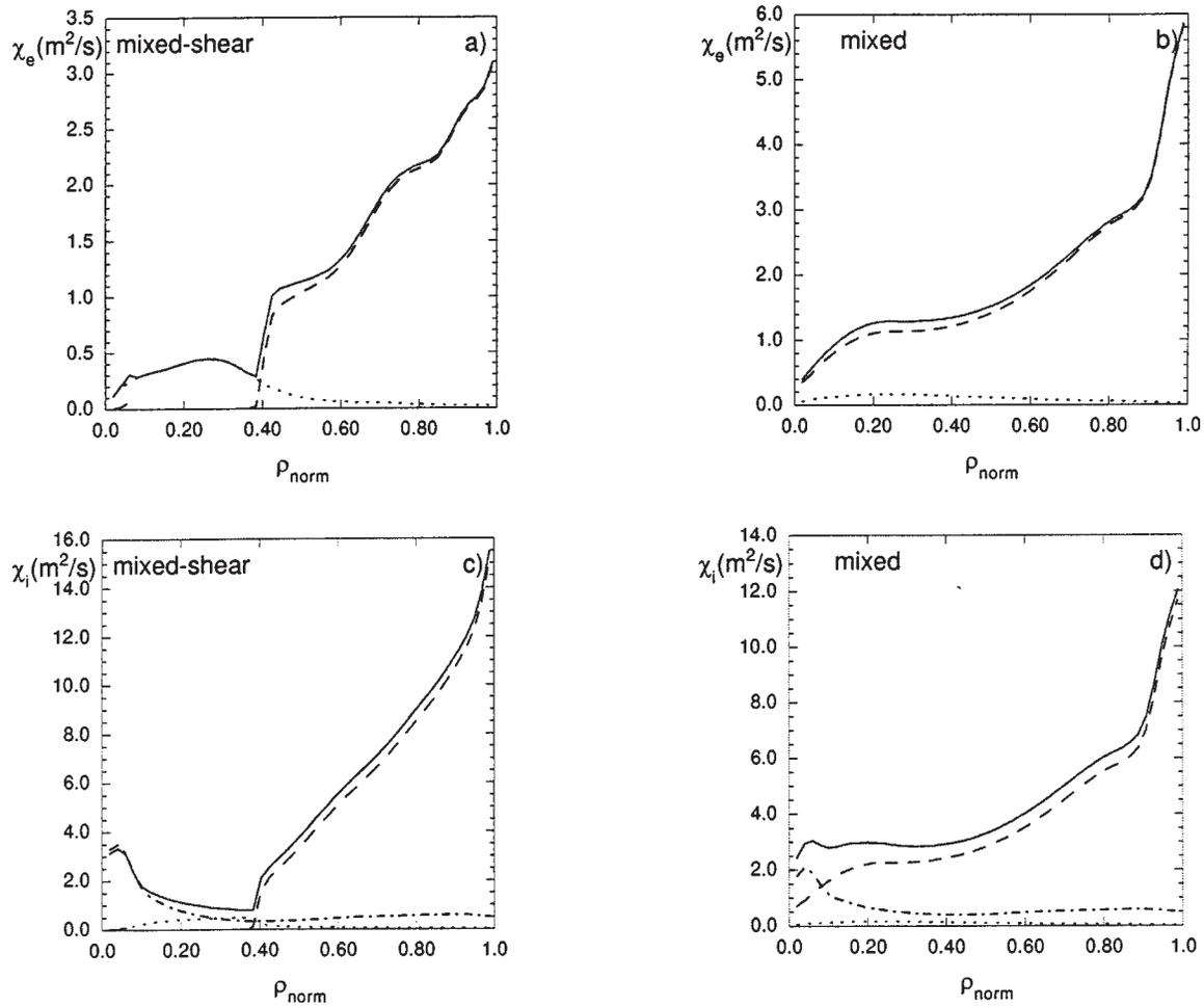
FIG. 12. Total (solid curves), Bohm (dashed curves), gyro-Bohm (dotted curves) and ion neoclassical (chain curves) thermal diffusivity radial profiles for (a, b) electrons and (c, d) ions for the same discharge as Fig. 10. The label ‘mixed shear’ refers to the diffusivity model proposed in this article, whereas the label ‘mixed’ refers to the model proposed in Ref. [12].
