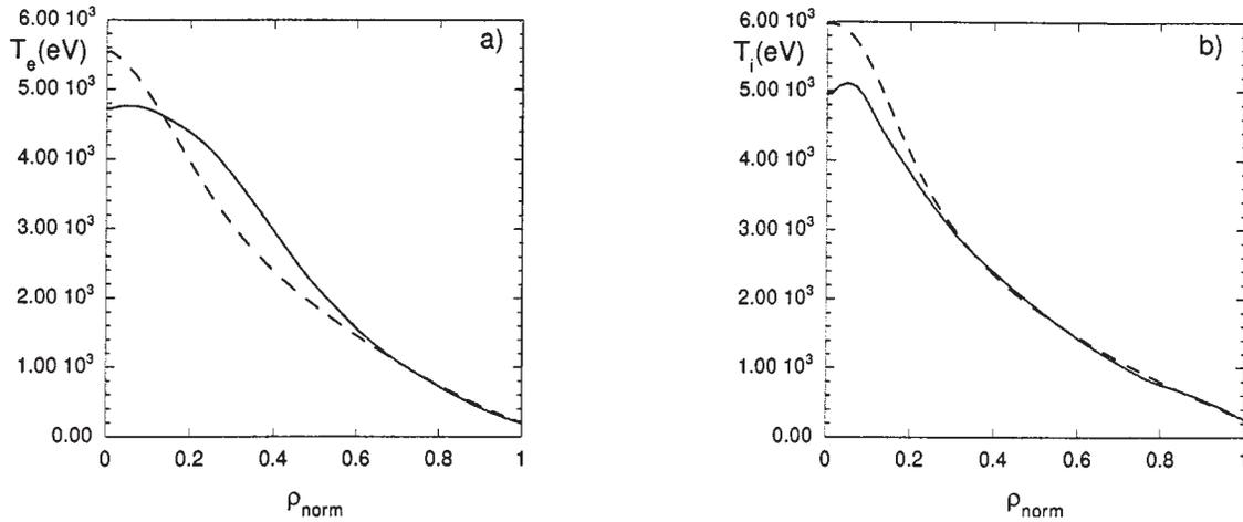
FIG. 1. Experimental (solid curves) and computed (dashed curves) electron (a) and ion (b) temperature profiles for JET discharge 19649 at  $t \simeq 50$  s.
