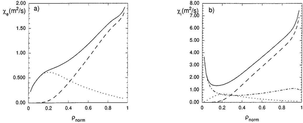
FIG. 5. Total (solid curves) electron (a) and ion (b) thermal diffusivity radial profiles and Bohm (dashed curves), gyro-Bohm (dotted curves) and ion neoclassical (chain curve) contributions for the same discharge as Fig. 3.
