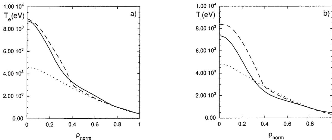
FIG. 10. Experimental (solid curves) and computed (dashed curves, mixed, shear dependent model proposed in this article; dotted curves, mixed model proposed in Ref. [12]) electron (a) and ion (b) temperature profiles for JET discharge 17749 at  $t \simeq 44.6$  s.
