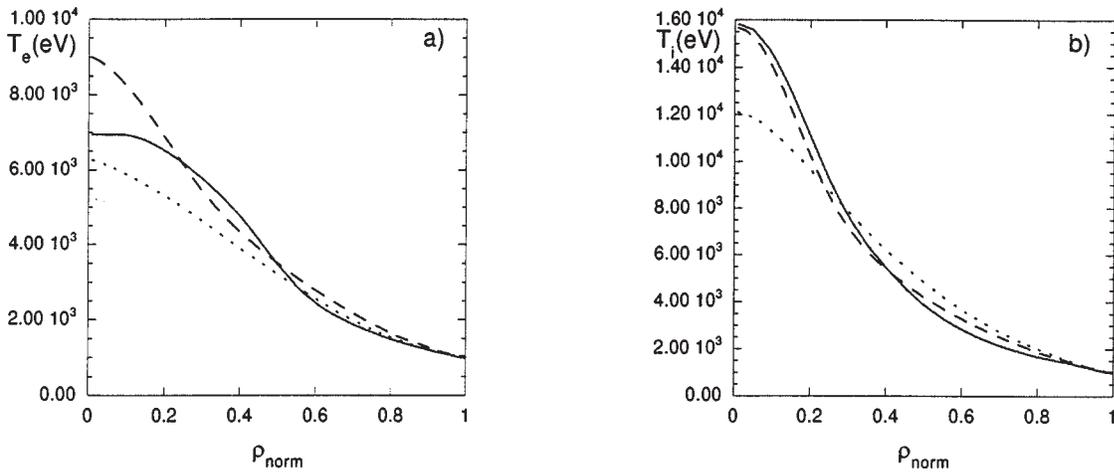
FIG. 13. Experimental (solid curves) and computed (dashed curves, mixed, shear dependent model proposed in this article; dotted curves, mixed model proposed in Ref. [12]) electron and ion temperature profiles for JET discharge 18757 at  $t \simeq 52.9$  s.
