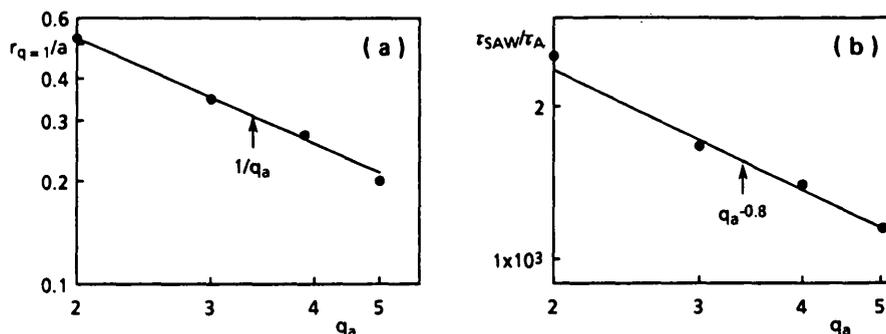
FIG. 2. (a)  $q = 1$  radius and (b) sawtooth repetition time  $\tau_{\text{saw}}/\tau_A$ , versus  $q_a$ . The values of the other parameters are defined in the text.
