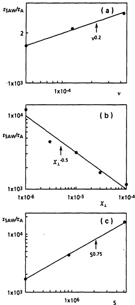
FIG. 1. Sawtooth repetition time  $\tau_{\text{saw}}/\tau_A$  versus: (a) perpendicular viscosity  $\nu$ , (b) perpendicular thermal diffusivity  $\chi_{\perp}$  and (c) Lundquist number  $S$ . The values of the other parameters are defined in the text.
