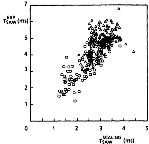
FIG. 3. Experimental sawtooth repetition time versus the scaling given by Eq. (8). Included are 299 shots of hydrogen, deuterium and helium gases; the linear correlation coefficient is  $r = 0.77$ . The open circles are data for 'non-saturated' discharges.
