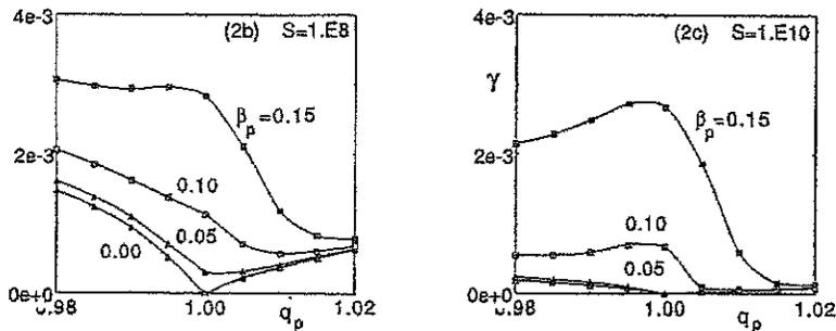
Figure 2. Resistive growth-rates for low-shear current profile and different  $\beta_{pol}$
