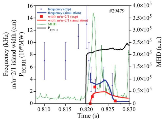
**Figure 10.** Time evolution of 2/1 mode, close to mode locking time, compared with the Rutherford model. Experimental frequency from Mirnov coils, MHD represents the  $B_\theta$  oscillations envelope and island width is determined from soft x-ray tomography.
