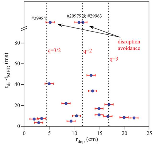
**Figure 9.** FTU power deposition scan: current quench delay versus  $r_{\text{dep}}$ ;  $t_{\text{dis}}$  = time of current quench;  $t_{\text{MHD}}$  = time of abrupt rise of MHD activity. The vertical axis is interrupted above 80 ms to accommodate discharges with disruption avoidance.
