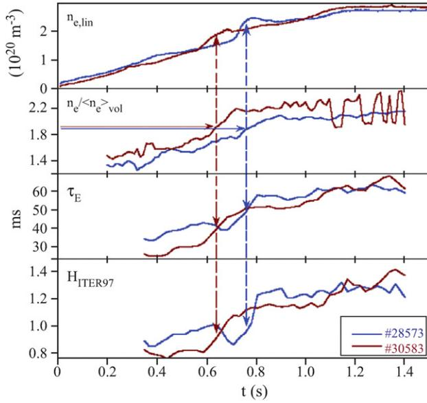
**Figure 1.** Time evolution of line averaged density, peaking factor, energy confinement time and  $H_{97}$  in two high-density discharges. In both cases, the transition to higher  $\tau_E$  occurs at the same value of  $n_{e0}/\langle n_e \rangle_{vol}$ .
