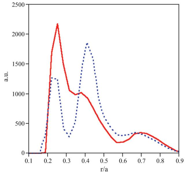
**Figure 4.** Fast electron radial profiles by inverted FEB camera data. Profiles are obtained integrating in phase ten fishbone oscillation periods: during positive half period (continuous curve) and during negative half period (dotted curve). Energy range 40–60 keV.
