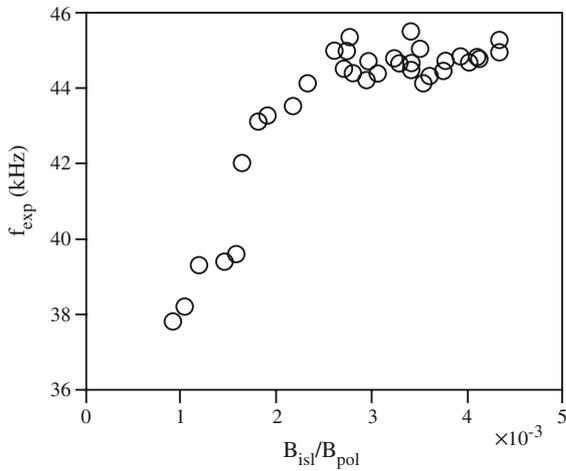
**Figure 7.** Mode frequency versus magnetic island amplitude observed in FTU shot 25877.
