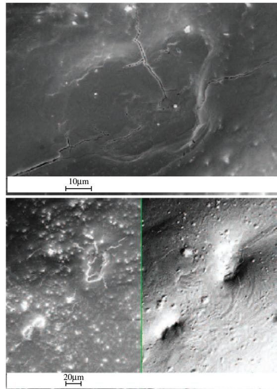
**Figure 11.** SEM analysis of the probe surface exposed to the FTU plasma. The scales indicated are  $10 \mu\text{m}$  in the upper figure, taken by secondary electron detector (SED) and  $20 \mu\text{m}$  for the lower figure, where SED (left) and electron back scattering (EBS) (right) images are compared for the same probe area.
