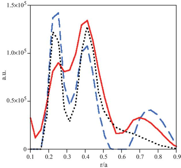
**Figure 5.** Fast electron radial profiles by inverted FEB camera data. Profiles are obtained with 3 ms integration window sliding across the mode: before the maximum of the mode (dashed line), after the maximum (full line) and at the end of the mode (dotted line). Energy range 40–60 keV.
