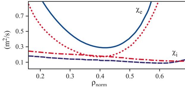
**Figure 2.** Electron and ion thermal conductivity for shot #28573 before and after the increase in the volume density peaking factor. Electrons: continuous line before density peaking, dotted line after; ions: dashed line before, dashed-dotted line after.
