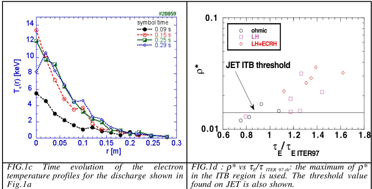
FIG.1c Time evolution of the electron temperature profiles for the discharge shown in Fig.1a
