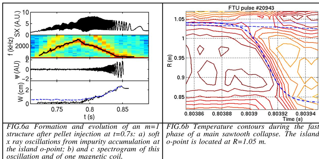
FIG.6a Formation and evolution of an  $m=1$  structure after pellet injection at  $t=0.7s$ : a) soft x ray oscillations from impurity accumulation at the island o-point; b) and c) spectrogram of this oscillation and of one magnetic coil.
