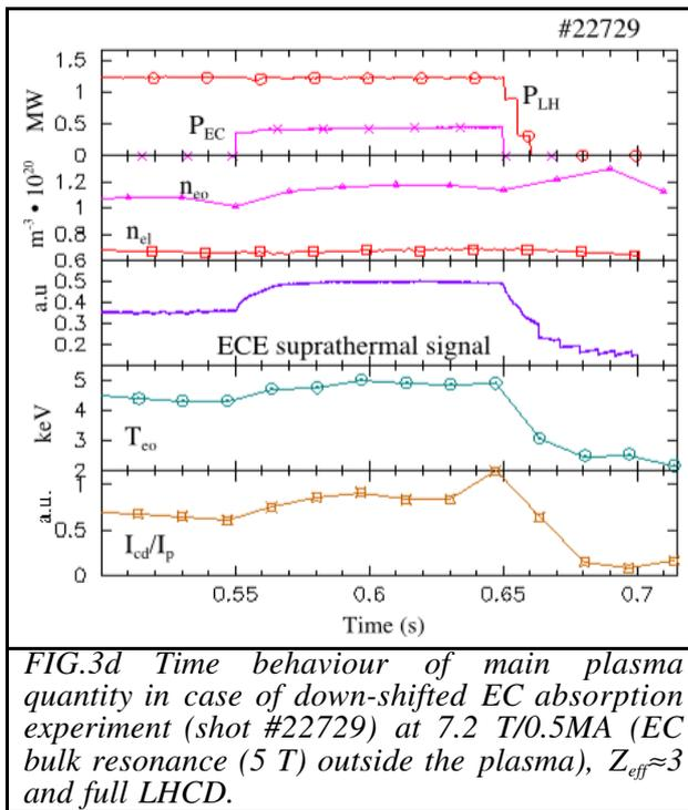
FIG.3d Time behaviour of main plasma quantity in case of down-shifted EC absorption experiment (shot #22729) at 7.2 T/0.5MA (EC bulk resonance (5 T) outside the plasma),  $Z_{eff} \approx 3$  and full LHCD.
