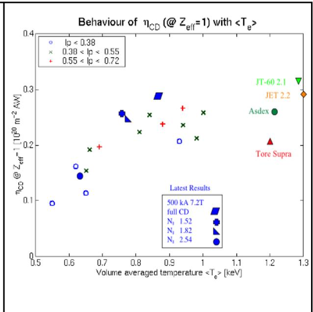
FIG.3c LHCD efficiency vs. average electron temperature.
