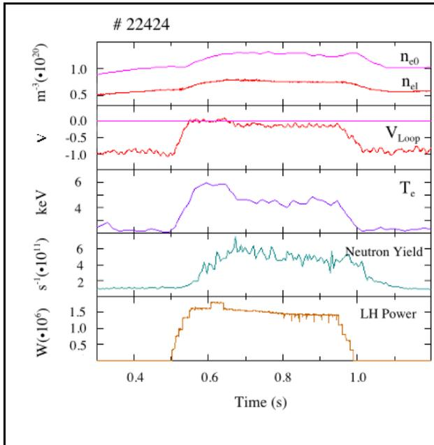
FIG 3b Full LHCD discharge at ITER relevant densities.
