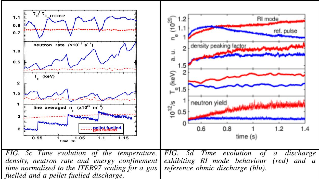
FIG. 5c Time evolution of the temperature, density, neutron rate and energy confinement time normalised to the ITER97 scaling for a gas fuelled and a pellet fuelled discharge.
