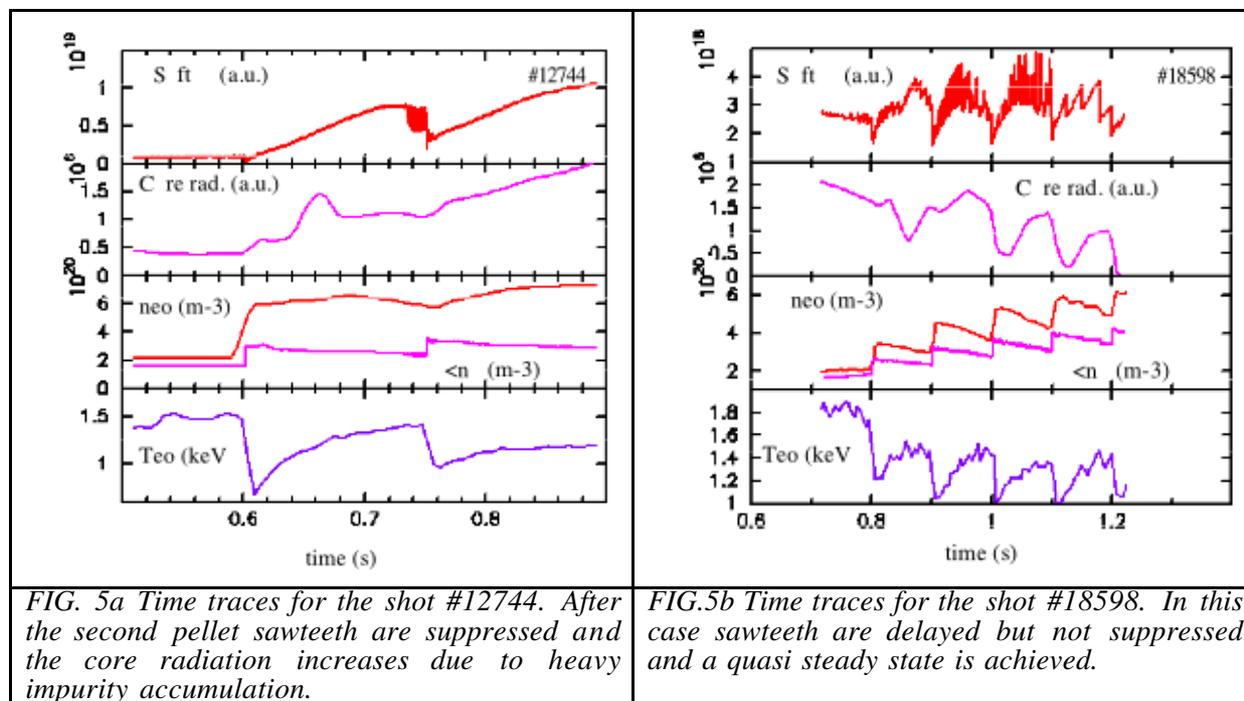
FIG. 5a Time traces for the shot #12744. After the second pellet sawteeth are suppressed and the core radiation increases due to heavy impurity accumulation.
