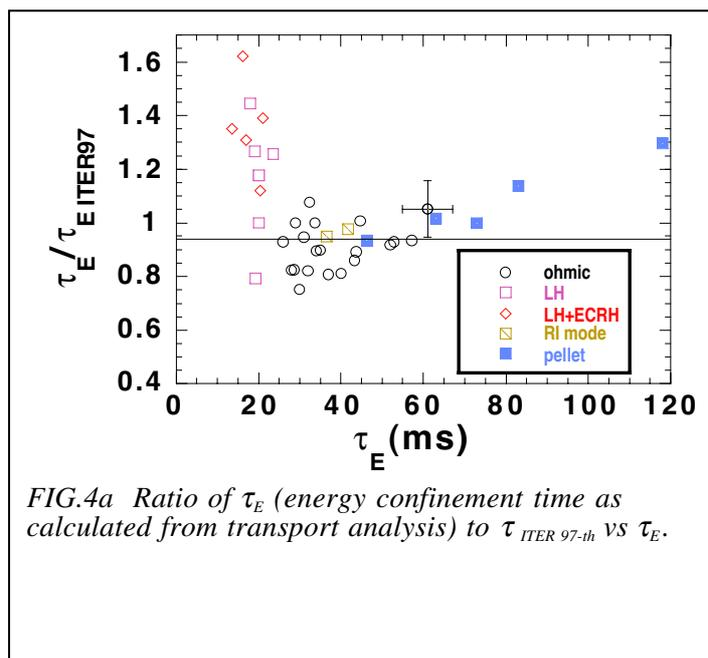
ohmic and L-mode discharges are generally in agreement with the ITER97 L-mode scaling. Discharges with an ITB have an energy confinement time up to 1.6 time the ITER97 scaling. The pellet discharges exhibit a time averaged confinement slightly above the ITER97 scaling, whereas gas fuelled discharges exhibit a confinement lower than the ITER97 scaling. Transient phases with enhancement factors up to 1.3 are observed but with the enhanced phase lasting less than one  $\tau_E$ .
