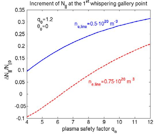
**Figure 5.** Relative increment of the launched  $N_{||}$  for an LH wave injected in FTU from the equatorial plane (according to [29]) as a function of the safety factor at the edge for two different plasma densities.
