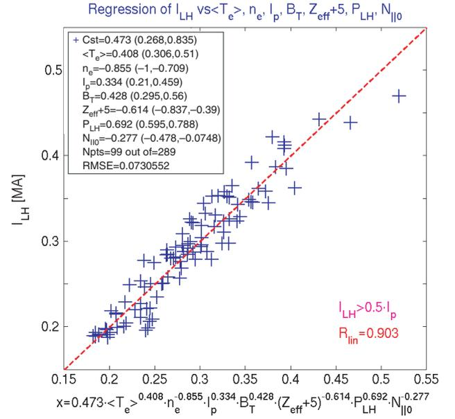
**Figure 3.** Multiple linear regression analysis for the amount of LH driven current. Only discharges with  $Z_{\text{eff}} < 6$  and  $I_{\text{LH}}/I_p > 50\%$  are considered. Units are  $T_e$  (keV),  $n_e$  ( $10^{20} \text{ m}^{-3}$ ),  $I_p$  (MA),  $B_T$  (T),  $P_{\text{LH}}$  (MW).
