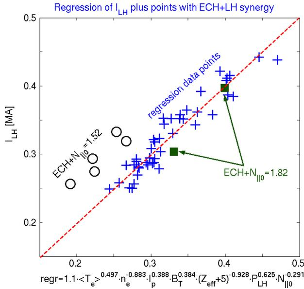
**Figure 9.** Total driven current in discharges with EC + LH waves and  $B_{T0} = 7.1$  T. Synergy, i.e. a substantial enhancement of  $I_{LH}$  with respect to the discharges in figure 2 (+), is visible only for  $N_{||0} = 1.52$  (O). The independent variable is the same as in figure 2.
