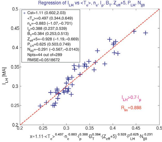
**Figure 2.** Multiple linear regression analysis for the amount of LH driven current. Only discharges with  $Z_{\text{eff}} < 6$  and  $I_{\text{LH}}/I_p > 70\%$  are considered. Units are  $T_e$  (keV),  $n_e$  ( $10^{20} \text{ m}^{-3}$ ),  $I_p$  (MA),  $B_T$  (T),  $P_{\text{LH}}$  (MW).
