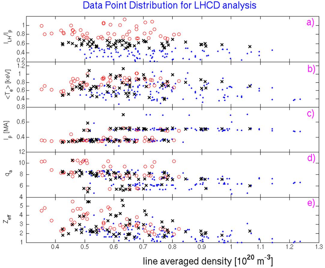
**Figure 1.** Distribution of the points in the FTU database for LHCD assuming the line averaged density as the free parameter. The analysis has been limited to discharges with  $Z_{\text{eff}} < 6$  and either with more than 70% of LH driven current (O) or extended also to  $50\% < I_{\text{LH}}/I_{\text{p}} \leq 70\%$  (x). The dots ( $\cdot$ ) refer to all the other discharges.
