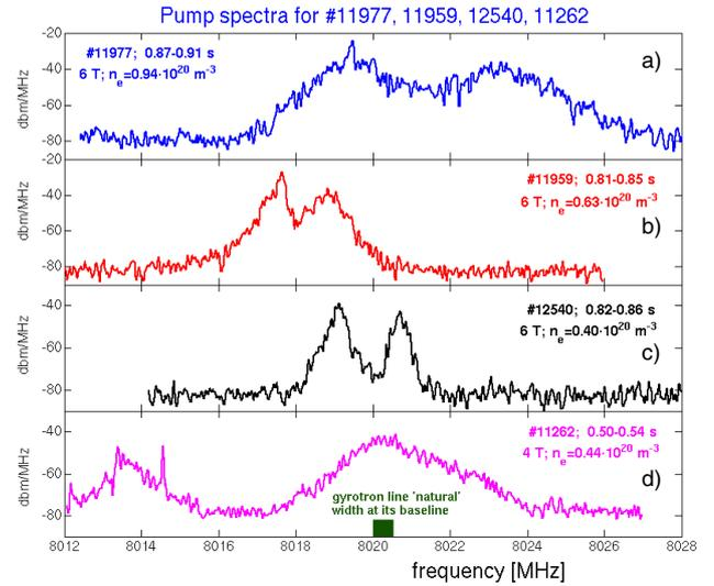
**Figure 7.** Frequency spectra around the pump frequency for two LH gyrotrons firing simultaneously into FTU. Three different plasma densities and two magnetic fields are considered. The spectral broadening clearly increases with  $\bar{n}_e$  and decreases with  $B_T$ . The natural width of the main gyrotron emission line is shown as a full box on the bottom frame.
