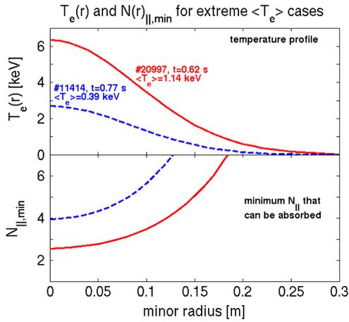
**Figure 6.** Profiles of  $e^-$  temperature (upper) and of the minimum absorbed  $N_{\parallel}$  (lower) for an LH wave in the two extreme cases in terms of  $\langle T_e \rangle$  of the data set analysed. Less  $N_{\parallel}$  upshift and hence more prompt absorption occurs in the hotter plasma case.
