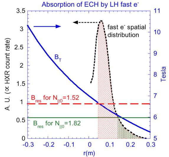
**Figure 10.** Distribution of the fast electron tails along the FTU minor radius, in arbitrary units. It is assumed proportional to the HXR perpendicular emission profile. The allowed interaction regions with EC waves are shown as shadowed areas, with dashes for the case  $N_{||0} = 1.52$  and lines for  $N_{||0} = 1.82$ .
