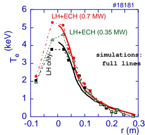
FIGURE 2 — #18181, electron temperature profiles. Experiment: symbols. a) LH only phase (squares), b)  $P_{ECH}=0.35$  MW, triangles; c)  $P_{ECH}=0.7$  MW, dots. Computation: full lines (cases a) and c))
