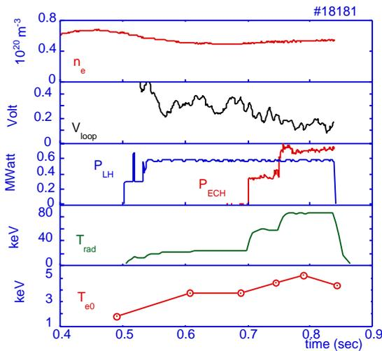
FIGURE 1. Shot 18181,  $B_T=7.2$ , time evolution of 1) line density; 2) loop voltage; 3) coupled LH and ECH power, 4) ECE emission along a central chord; 5) central electron temperature
