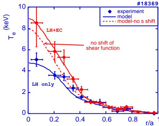
**FIGURE 3.** Electron temperature profiles for shot 18369. Solid symbols: experiment; lines: computation.  $P_{LH}=0.65$  MW,  $P_{ECH}=0.36$  MW. In the LH+ECH case the shear variable  $s$  has been shifted by 0.5, i.e  $s \rightarrow s-0.5$ . The dashed line refers to unshifted  $s$ .
