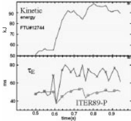
**Figure 5.** Evolution of the internal energy and confinement time as compared with the ITER-89P values for discharge FTU 12744.
