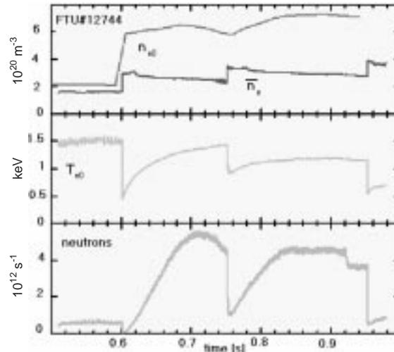
**Figure 1.** Time traces of the most significant parameters of discharge FTU 12744,  $B = 7 \text{ T}$ ,  $I = 0.8 \text{ MA}$ ,  $q = 4.7$ . Pellets were injected at 0.65, 0.75 and 0.95 s.
