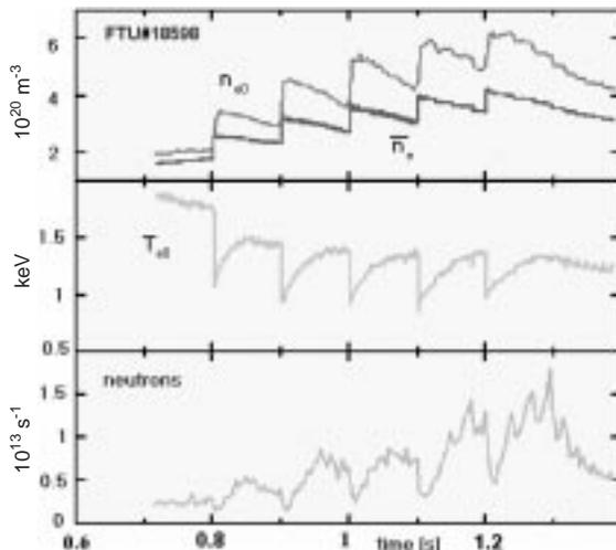
**Figure 2.** Time traces of the most significant parameters of discharge FTU 18598,  $B = 8$  T,  $I = 1.23$  MA,  $q = 3.3$ . Pellets were injected from 0.8 s at 100 ms intervals.
