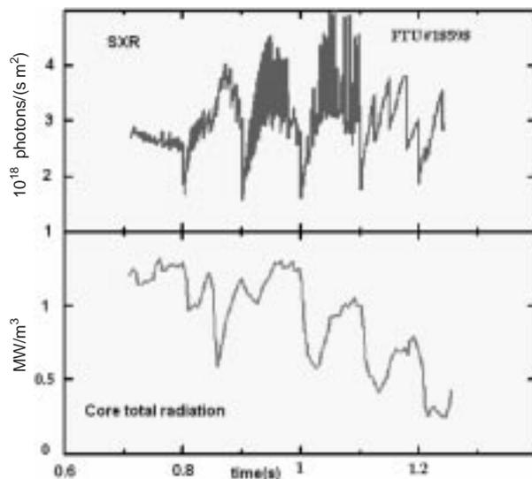
**Figure 8.** Soft X ray emission along a central chord and total core radiation in discharge 18598.
