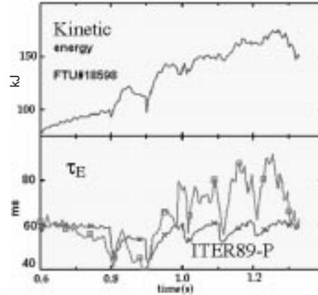
**Figure 6.** Evolution of the internal energy and confinement time as compared with the ITER-89P values for discharge FTU 18598.
