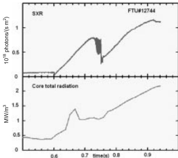
**Figure 7.** Soft X ray emission along a central chord and total core radiation in discharge FTU 12744.
