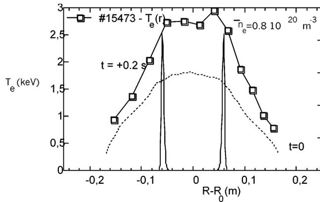
**Figure 3.** At high electron density, off-axis ECRH ( $P_{\text{abs}}$  from beam-tracing is shown, a.u.) and e-i thermal exchange produce hollow temperature profiles.
