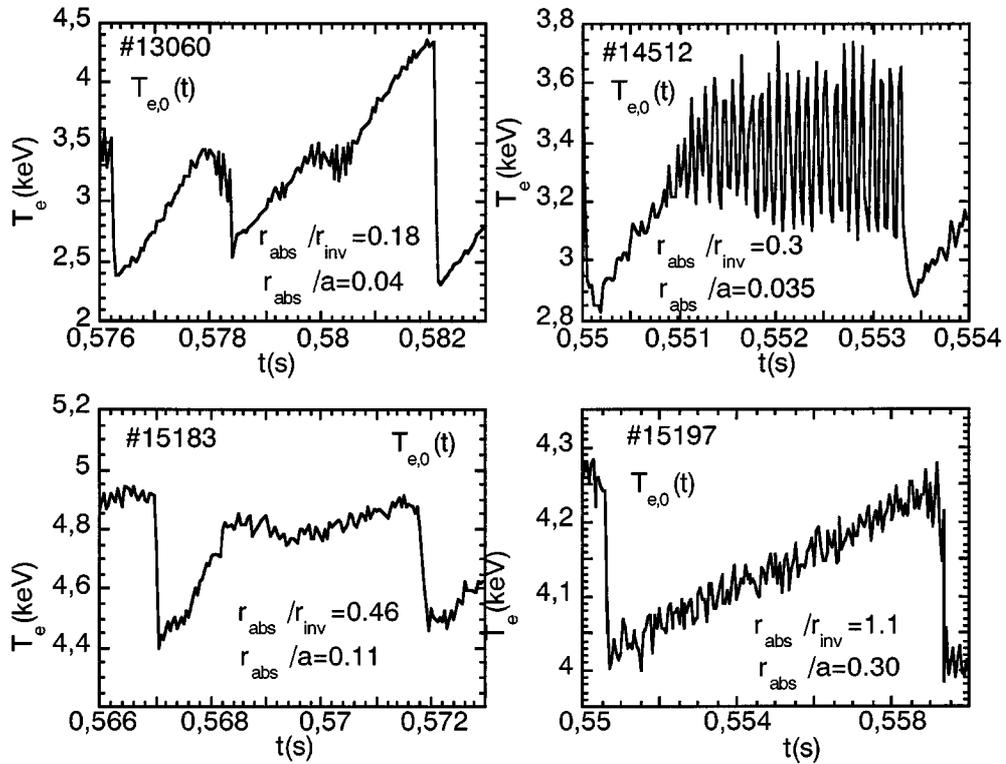
**Figure 16.** Central temperature with ECRH at different positions with respect to the 1/1 MHD island. The sawtooth shape varies very much with position, until a regular sawtooth reappears as the absorption is shifted well outside the inversion radius.
