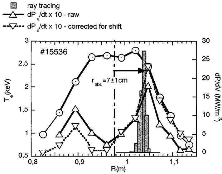
Figure 4. The estimate of the absorbing layer from beam-tracing agrees with the position where the heating rate at ECRH-ON is faster.
