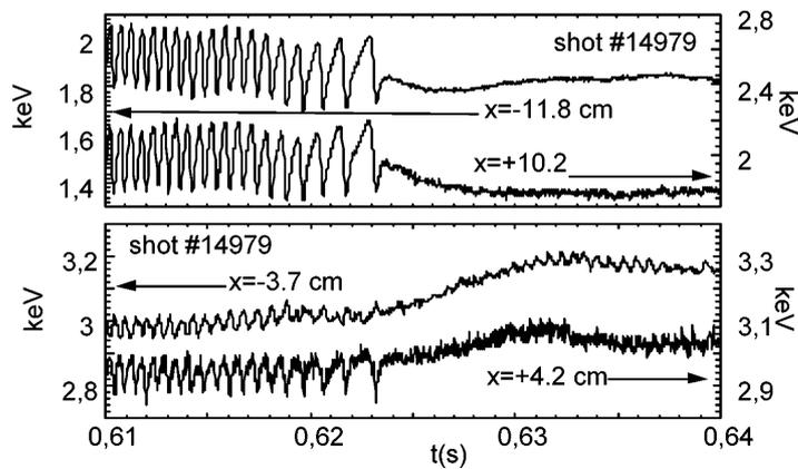
**Figure 9.** Toroidal geometry may couple the 2/1 and 1/1 modes, as shown by temperature fluctuations at  $r \approx r_{q=2}$  (top) and at  $r \approx r_{q=1}$  (bottom). When 2/1 locks to the walls, 1/1 continues free but at a lower amplitude.
