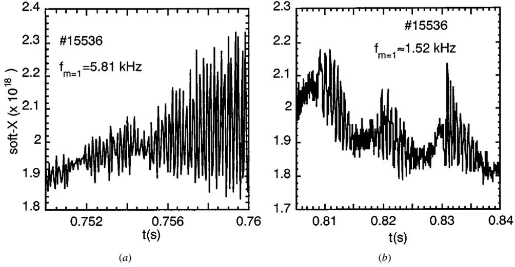
**Figure 11.** In shot #15536  $m = 1$  instability, after transient stabilization, persists for the whole ECRH pulse (cf figure 6). The frequency is higher when the mode reappears after stabilization (a) and  $r_{q=1}$  is small, than at later times (b) when the mode is close to reconnection.
