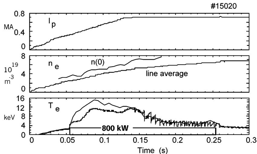
**Figure 1.** Plasma current, electron density (line average and peak), and electron temperature with central ECRH at 800 kW during current ramp-up.
