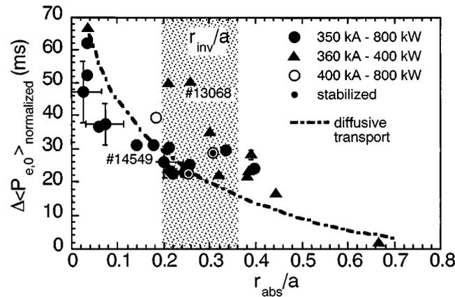
**Figure 14.** Central heating versus the position of the absorption layer. The pressure increase is normalized to  $P_{\text{ECRH}}$  and to the plasma volume. Dots mark the discharges with full  $m = 1$  stabilization with off-axis ECRH (at 400 kW, 400 kA). The dashed line shows the trend expected with smooth diffusivity (from power balance at 800 kW).
