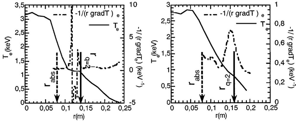
**Figure 12.** Shoulders are developed on the temperature profile by 2/1 MHD islands, which depend on the island width. The enhanced thermal diffusivity at  $r \approx r_{q=2}$  is visible also in discharges apparently free of macroscopic  $m = 2$  oscillations (right). In the large island (left) the temperature may not be flat, but slightly increasing towards the outward edge.
