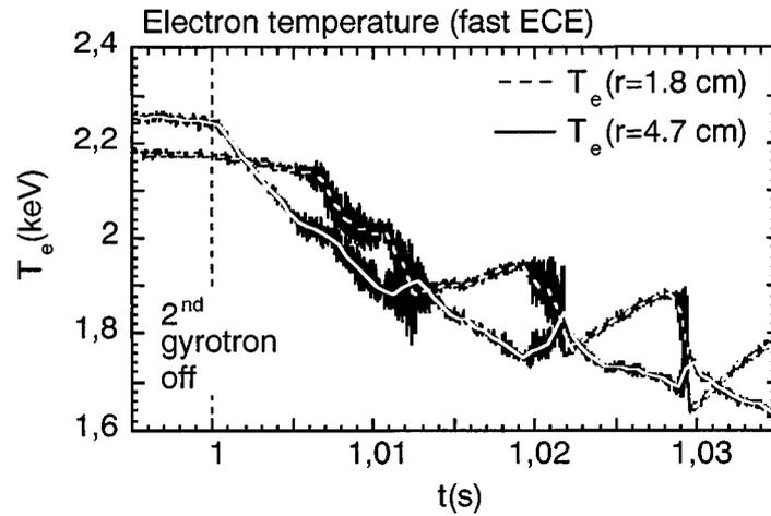
**Figure 7.** Electron temperature (fast ECE measurements) at two radial points close to the plasma centre. As the  $1/1$  mode reappears after stabilization, core confinement is degraded.
