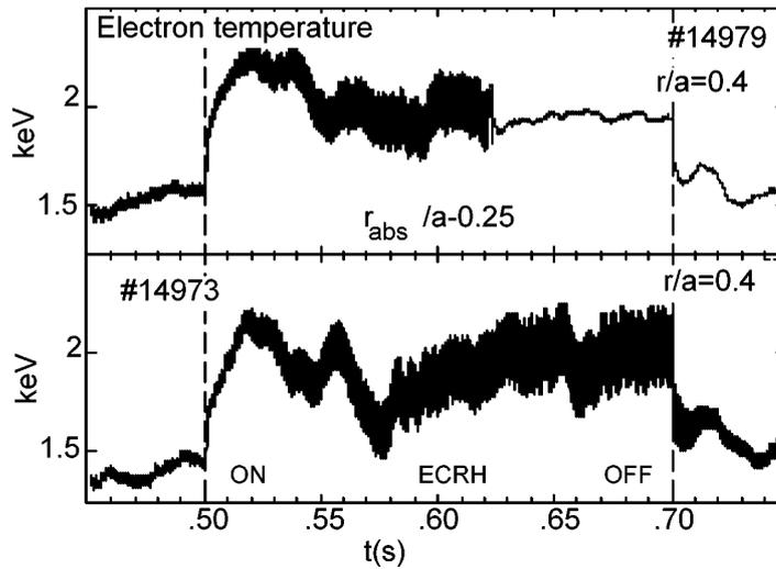
**Figure 8.** ECRH at  $r_{\text{abs}} \approx r_{\text{inv}}$  may further destabilize pre-existing tearing modes  $m = 2, n = 1$ . The figure shows the electron temperature (ECE diagnostic) at  $r \approx r_{q=2}$ . The mode may eventually become locked (top) by the wall braking torque (cf figure 9), or may continue to exist for the whole pulse length depending on its frequency.
