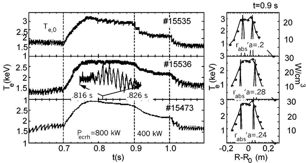
**Figure 6.** Central electron temperature (left) and temperature profiles at steady-state (right), for three discharges with ECRH aiming at  $m = 1, n = 1$  mode stabilization. Within a shift  $\approx 2$  cm (8% of the minor radius), all possible effects are observed, from sawtoothing to a fully stabilized plasma.
