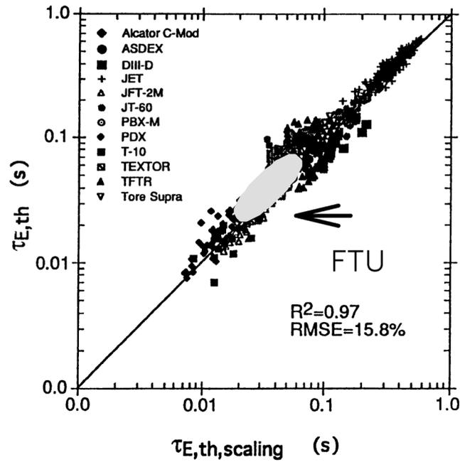
Figure 5. The global energy content with ECRH at steady-state scales in fair agreement with ITER L-mode scaling laws. FTU data with ECRH are compared in the figure with ITER97 scaling [22].
