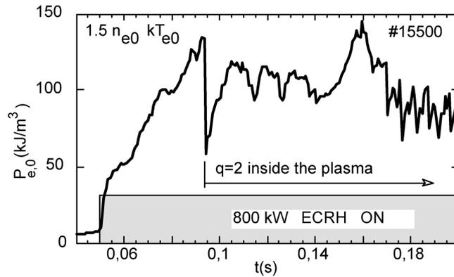
**Figure 13.** Peak pressure evolution during current ramp-up with central ECRH. The appearance of a rational- $q$  surface is marked by a strong internal disruption due to the double tearing mode. After 2/1 disruption ( $\approx 0.1$  s), the central energy density does not fully recover.
