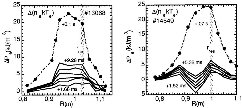
**Figure 15.** Pressure profile evolution after ECRH switching-ON. As expected from diffusive transport, the profile for #14549 is hollow at the beginning and fills up at longer times. For #13068, the energy density profile is rapidly flattened, as if inward heat convection were active. Also, at steady-state the energy content is the same for the two discharges, but  $P_{\text{ECRH}}$  in #14549 is twice than in #13068.
