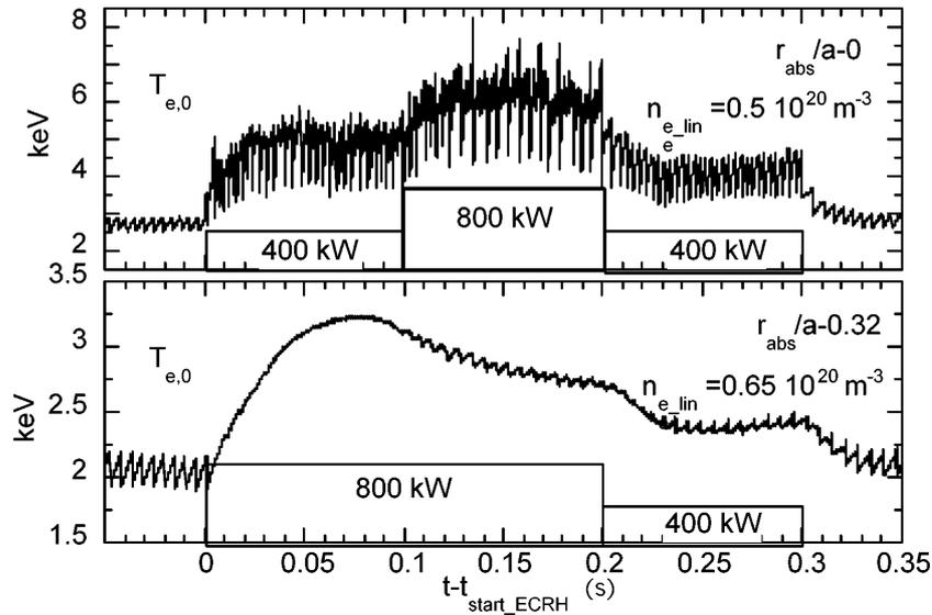
**Figure 2.** Peak electron temperature for on-axis (top) and off-axis (bottom) ECRH at current flat-top. Sawteeth are larger and faster when heating at the centre, and may be stabilized when EC power is absorbed at about the inversion radius.
