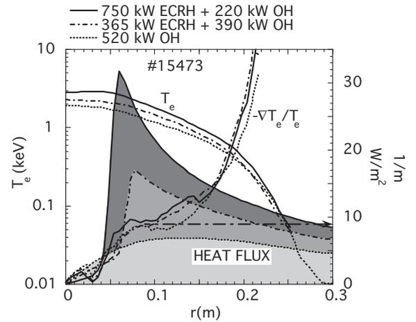
**Figure 1.** Electron temperature, gradient length and heat flux versus radius for different levels of ECRH intensity. The electron temperature gradient length does not increase with stronger heating. Note that the major radius being  $R \approx 0.98$  m,  $1/L_T$  can be directly used for normalized comparisons.
