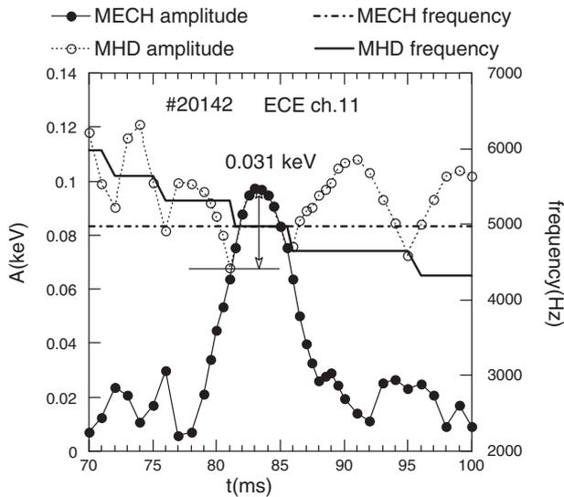
**Figure 15.** The figure shows the ability of the analysis of MECH data at high modulation frequency to discriminate true modulation from MHD effects. Closed circles correspond to the peak amplitude in the FFT spectrum at the modulation frequency, while open circles correspond to the MHD component. When the two frequencies are close, beating between MHD and MECH components appears.
