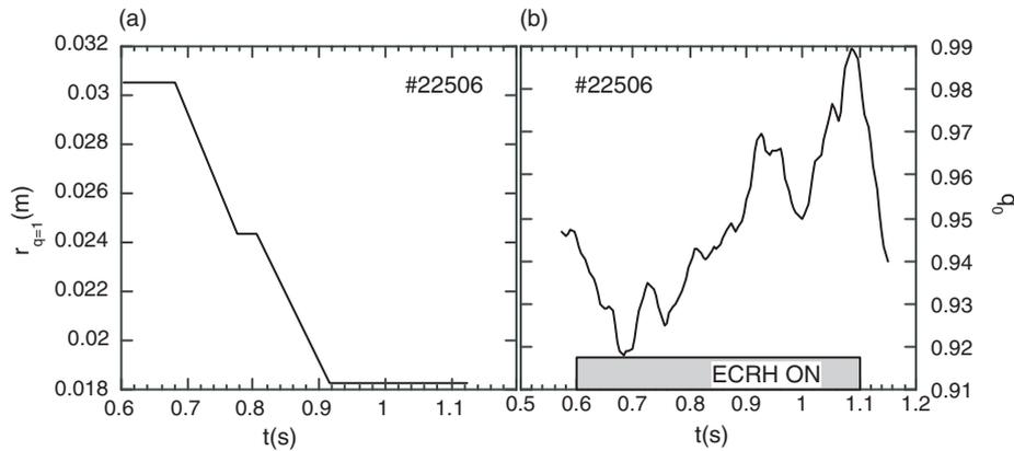
**Figure 8.** (a) shows the evolution in time of the  $q = 1$  radius, (b) the central  $q$  is shown versus time. The  $q$ -profile is estimated by equilibrium reconstruction, conditioned by power balance analysis.
