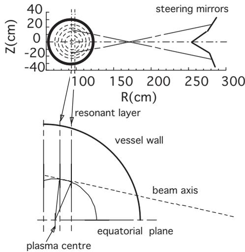
**Figure 17.** The scheme of the relative position of EC beams axis and plasma column is shown in the figure. With this arrangement, although a toroidal field scan moves the resonant layer and the ECE grid of measuring points along the minor radius, the EC absorption remains peaked on the same magnetic surface. Therefore, the ECE grid moves with respect to the ECH absorption.
