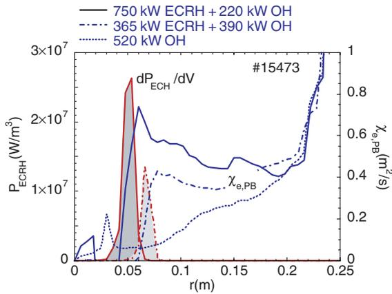
**Figure 2.** In order to maintain the temperature gradient length  $L_T$  constant also during ECRH, and smooth across the absorption layer, the electron thermal diffusivity  $\chi_e$  develops a step at a deposition radius  $r_{\text{dep}}$ , larger with stronger heating.
