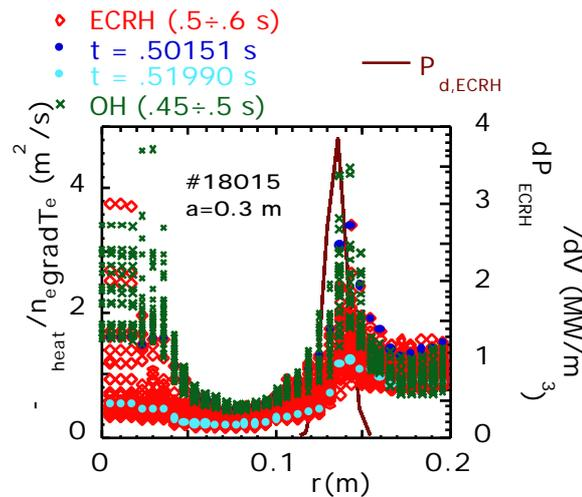
Fig.6  $\chi_{e,eff}$  vs. minor radius in the ohmic phase (green x) and during TM stabilization (red diamonds). ECRH profile closely overlaps the island (high  $\chi_{e,eff}$  region at 0.14 m).
