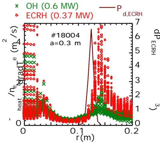
Fig.11  $\chi_{e,eff}$  vs. minor radius in the ohmic phase (green x) and during ECRH (red diamonds). ECRH profile is shifted 3 cm inward with respect to the island (high  $\chi_{e,eff}$  region at 0.14 m). In this case TM is further destabilized and the island width is further increased.
