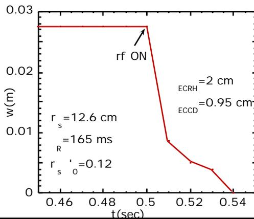
*Fig.7 Island width evolution estimated by using a Rutherford type relation between growth rate and stabilizing/destabilizing factors, including the term due to EC induced helical currents (by heating and current drive). Key parameters are equal to the experimental values. Estimate is close to experiment.*
