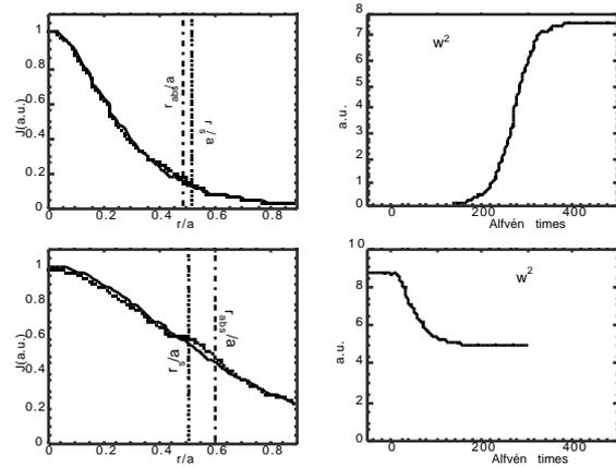
*Fig.8 Estimate of the island width evolution determined by a local symmetric perturbation of the current density profile, close to the one expected during experiments on TM control with ECRH. It shows that  $\Delta'$  changes may contribute to TM suppression, in addition to helical currents effects.*
