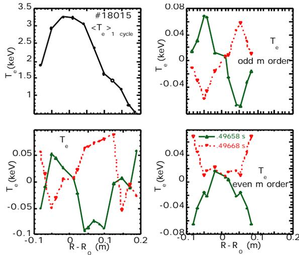
Fig.2 Radial profile of electron temperature (top-left) fluctuations (bottom-left) shows that an odd mode (top-right), central, and an even mode (bottom-right) coexist. The two modes are tightly linked, their frequency being exactly the same.
