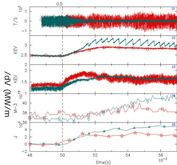
Fig.12 Shot #18004 and #18015 are compared. In #18004 absorption is at  $r_{abs}/a=0.46$ , 3 cm and stabilization fails. Top to bottom: Mirnov signals,  $T_{e,ECE}$  at center and half radius, central line density, global energy increase. Core confinement improves with TM stabilization.
