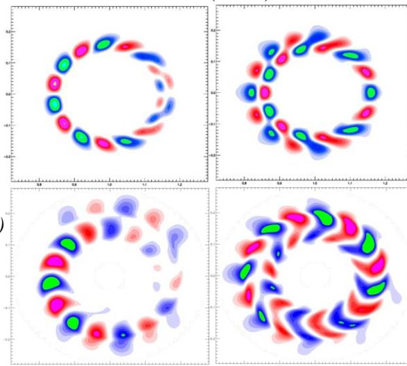
**Fig. 5** GTC simulation of  $n=5$  TAE excitation by an antenna (upper panels) and fast ions (lower panels). Left column is the contour plots of vector potential ( $A_{||}$ ) and right column is electrostatic potential ( $\phi$ ).
