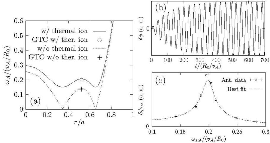
**FIG. 2.** Antenna excitation of  $n = 4$ ,  $m = 7$  RSAE with kinetic thermal ions using GTC. (a)  $m = 7$  Alfvén continua and eigen-frequencies obtained from GTC simulations, with and without thermal ions. (b) Time history of electrostatic potential  $\delta\phi$  for antenna frequency  $\omega_{\text{ant}} = 0.195v_A/R_0$  showing saturation of the mode. (c) Saturated  $\delta\phi$  amplitude versus antenna frequency and best fit to estimate the RSAE damping rate.
