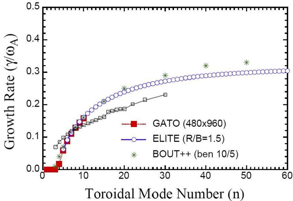
**Fig. 8:** GTC simulation of ideal ballooning mode: linear growth rate as a function of  $n$ , compared to the results from several fluid codes in Ref. [25].
