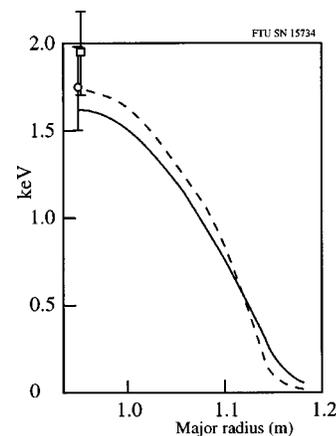
FIG. 3. Neoclassical ion temperature profile and central ion temperature obtained from He-like spectroscopy of iron spectroscopy, at different times: before (continuous curve and circle, respectively) and during IBW power injection (dashed curve and square, respectively).
