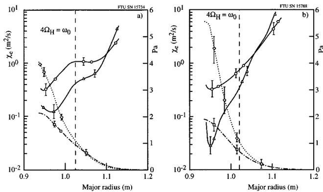
FIG. 4. Electron thermal diffusivity profile from transport analysis, before (circles) and during IBW injection (triangles), for coupled IBW power 0.25 MW (a) and 0.35 MW (b). The bars show the error produced by the experimental kinetic profiles and the effective ion charge. The respective measured pressure profiles are shown for comparison.
