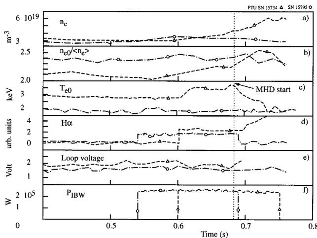
FIG. 1. Comparison of the time evolution of the main plasma parameters during injection of the same IBW power (0.25 MW), in plasma shots with resonant magnetic field:  $B_T=7.9$  T ( $I_p=330$  kA) (triangles), and with  $B_T=5.9$  T ( $I_p=240$  kA) (circles). Line averaged plasma density (a), density profile peaking  $n_{e0}/\langle n_e \rangle$  (b), central electron temperature from ECE (c),  $H\alpha$  emission from the outer plasma edge (d), loop voltage (e), IBW power (f).
