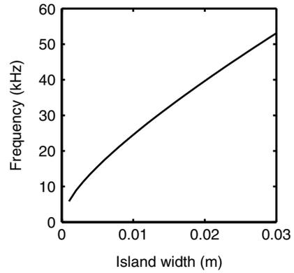
**Figure 7.** Frequency of discrete Alfvén modes from equation (5) as a function of island size. Plasma parameters are  $V_A = 1.7 \times 10^7$  m s<sup>-1</sup>,  $d_c = 1$  mm,  $\rho_S = 0.77$  mm,  $r_0 = 160$  mm,  $v_{ei} = 0.13$  MHz,  $k_{\perp} = 2/r_0$ ,  $q_0 = 2$ ,  $n_0 = 1$ .
