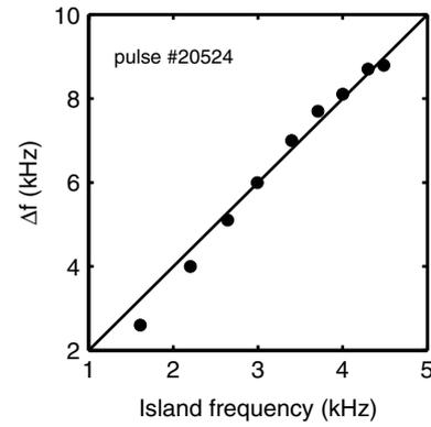
**Figure 2.** Frequency difference between the two dominant HF lines versus the island rotation frequency.
