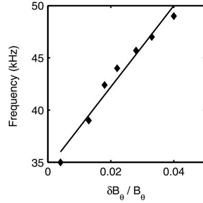
**Figure 4.** Frequency of the  $n = -1$  HF mode as a function of tearing mode oscillation amplitude; the latter is proportional to the squared island width.
