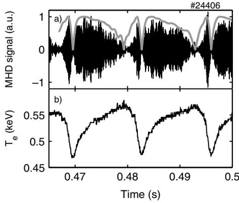
**Figure 3.** (a) HF signals (filtered with 42–53 kHz bandpass) from magnetic coil 5 ( $16^\circ$  above midplane) showing beat-waves structure. (b) Temperature oscillations from an ECE channel ( $R = 0.8$  m) close to the island position, showing (non-uniform) island rotation. The grey trace in (a) shows the envelope as expected from the phase of signal (b).
