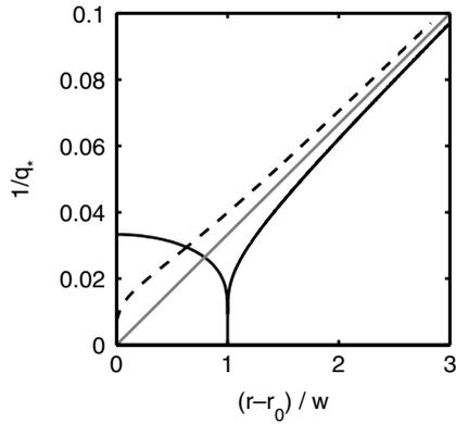
**Figure 6.** Radial profiles of the inverse helical  $q$  at  $\beta = \pi/2$  (---), separatrix at  $r = r_0$  and at  $\beta = 0$  (—, separatrix at  $r = r_0 + w$ ). Profiles are calculated for  $s = 1$  and  $n_0 = 1$ . The straight line in grey shows the no-island slope  $1/q_{\text{cyl}}$ .
