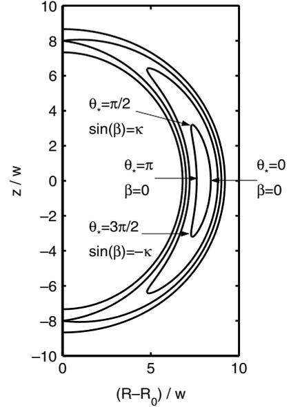
**Figure 5.** Schematic of  $m = 2$  island flux surfaces with normalized island width  $w/r_0 = 0.125$ , which is representative for the conditions of figure 3,  $r_0 = 16$  cm and  $w = 2$  cm. Contours are shown for  $\kappa = 0.4, 0.8, 1.0$  (the separatrix) and  $1.2$ . The  $z$  coordinate represents distance from the equatorial plane.
