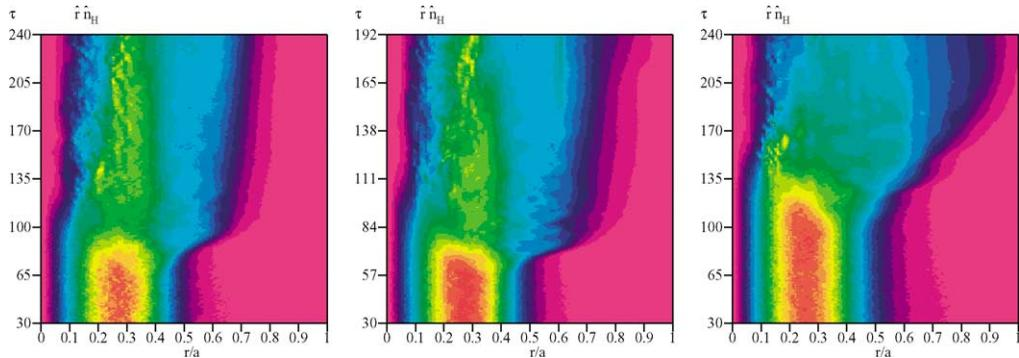
Fig. 6. Contour plot of the normalized line density,  $\hat{r}\hat{n}_H$ , of energetic ions in the  $(r/a, \tau)$  plane for the three low- $\beta_H$  ( $\beta_H(0) = 0.025$ ) cases: the deeply hollow  $q$ -profile case, with flat (left) or decreasing thermal-plasma density (center), and the moderately hollow  $q$ -profile case (right).
