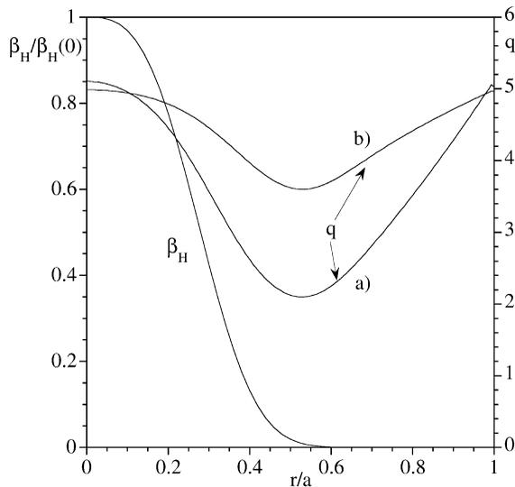
Fig. 1. The two different hollow  $q$  profiles and the initial  $\beta_H$  profile adopted in the simulations.
