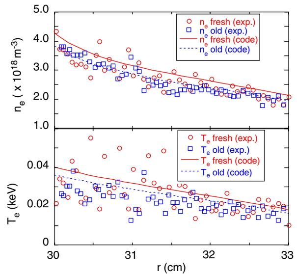
**Figure 9.** Experimental (symbols) and code (lines) radial profiles of electron density (first frame) and electron temperature (second frame) in the SOL plotted against the minor radius after a fresh boronization (#22871) and after an old boronization (#23186). For both discharges  $\bar{n}_e = 0.45 \times 10^{20} \text{ m}^{-3}$  and  $\theta = 240^\circ$  measured from the outer equatorial plane in the counter-clockwise direction.
