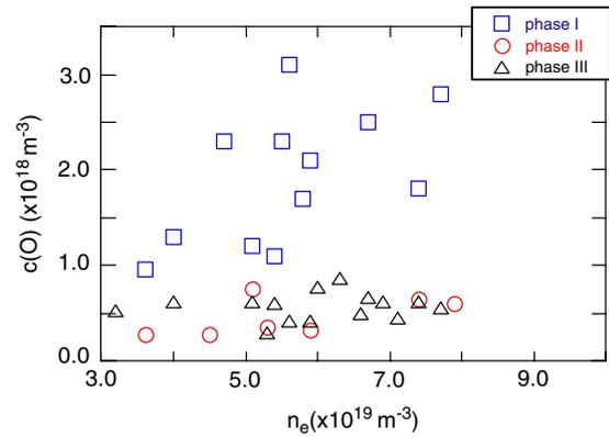
**Figure 5.** Oxygen concentration in the plasma as a function of the average electron density for the same discharges of figure 3. Very low values are also obtained after 500 discharges after boronization.
