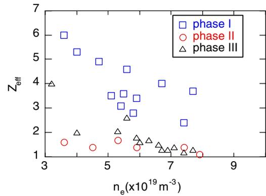
**Figure 4.** Experimental  $Z_{\text{eff}}$  against the average electron density before (phase I), immediately after (phase II) and at long time distance from boronization (phase III) for the same discharges of figure 3.
