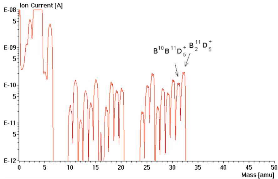
Figure 1. Mass spectrum of QMA during the boronization process.
