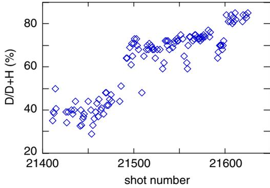
**Figure 6.** Ratio of deuterium to deuterium + hydrogen fluxes as a function of shot number starting from the first discharge after boronization (#21411).
