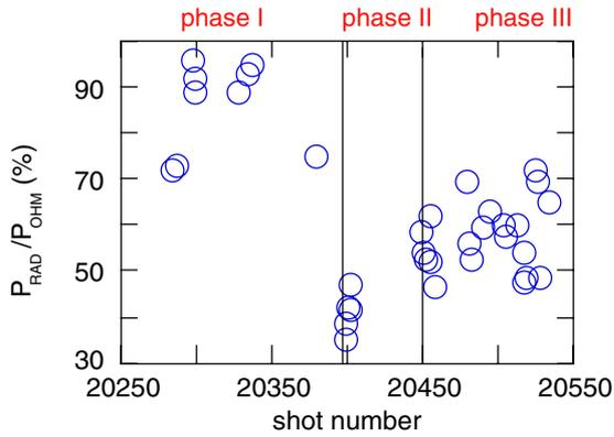
**Figure 3.** Fraction of the radiated power  $P_{\text{RAD}}$  to the ohmic power  $P_{\text{OHM}}$  (in per cent) as a function of the shot number for ohmic discharges with  $I_p = 0.5$  MA and  $\bar{n}_e = 0.3\text{--}0.8 \times 10^{20} \text{ m}^{-3}$ .
