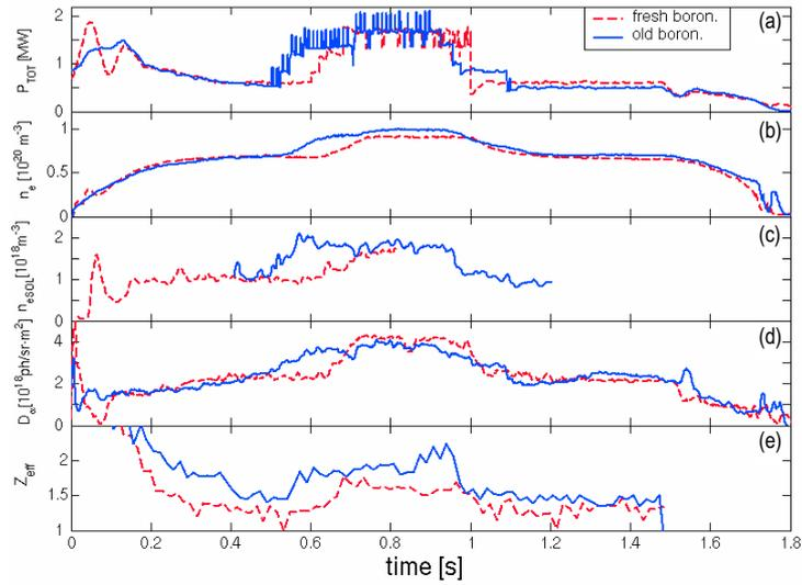
**Figure 12.** Temporal evolution of (a) total input power, (b) average electron density, (c) electron density in the SOL, (d)  $D_\alpha$  emission and (e)  $Z_{eff}$  value after a fresh boronization (#21470; - - -) and after an old boronization (#20739; —). For both discharges  $I_p = 0.5$  MA and  $P_{LH} = 1.65$  MW.
