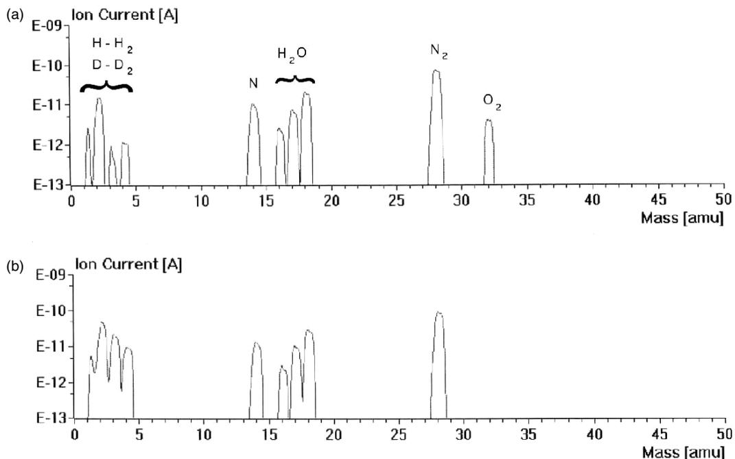
Figure 2. Mass spectra at cryogenic temperature (a) before and (b) during the experimental session. Oxygen disappears after a few plasma discharges.
