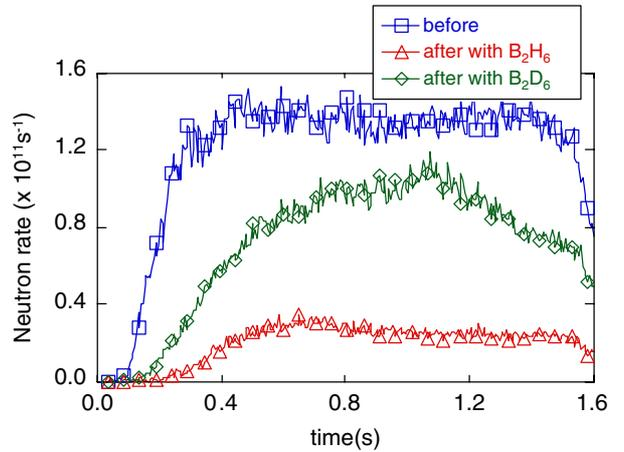
**Figure 7.** Comparison of neutron generation rate for three plasma discharges: the first one obtained before boronization (#20286), the second one after boronization with  $\text{B}_2\text{H}_6$  (#20401) and the third one after boronization with  $\text{B}_2\text{D}_6$  (#22862). In all the cases  $\bar{n}_e = 0.5 \times 10^{20} \text{ m}^{-3}$ ,  $I_{\text{p}} = 0.5 \text{ MA}$ ,  $B_{\text{T}} = 6 \text{ T}$ .
