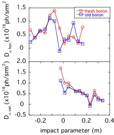
**Figure 10.**  $D_\alpha$  emission along horizontal and vertical chords plotted as a function of the impact parameter for wall conditions immediately after boronization (#22871) and at long time distance from boronization (#23186).
