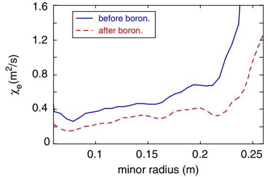
**Figure 8.** Radial profile of electron heat conductivity for two plasma discharges before (#20286) and after (#22864) boronization with  $\text{B}_2\text{D}_6$ .
