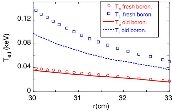
**Figure 11.** Predicted  $T_i$  and  $T_e$  radial profiles in the SOL for  $\vartheta = 240^\circ$  starting from the LCMS down to the wall position after a fresh boronization (#22871) and after an old boronization (#23186). For both discharges  $\bar{n}_e = 0.45 \times 10^{20} \text{ m}^{-3}$ ,  $I_p = 0.5 \text{ MA}$  and  $B_T = 6 \text{ T}$ .
