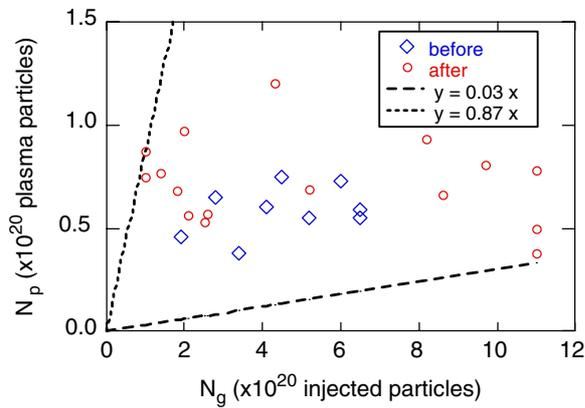
**Figure 13.** Plot of the total plasma particles  $N_p$  versus the total amount of injected particles  $N_g$ . The dotted lines define the range of  $N_p/N_g$  variation after boronization.
