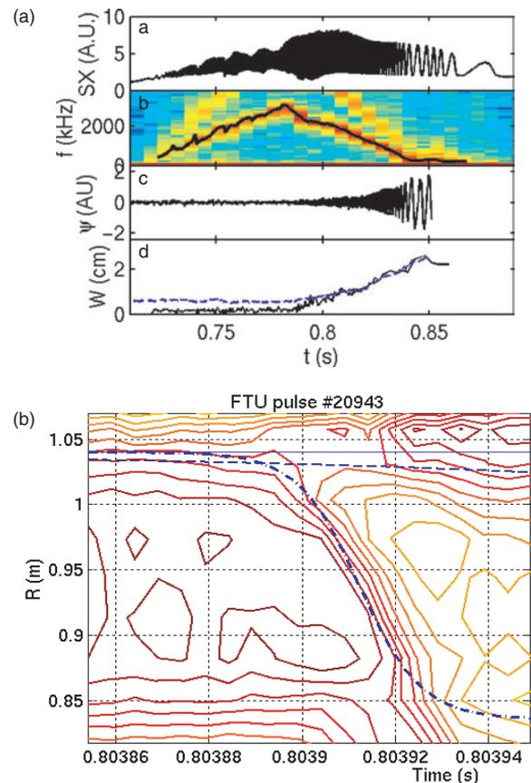
**Figure 6.** (a) Formation and evolution of an  $m = 1$  structure after pellet injection at  $t = 0.7$  s: (a) soft-x-ray oscillations from impurity accumulation at the island O-point; (b) spectrogram of this oscillation; (c) edge poloidal field oscillations; (d) island width evolution from ECE (black) and from magnetic coil (blue). (b) Temperature contours from ECE during the fast phase of a main sawtooth collapse. The island O-point is located at  $R = 1.05$  m.
