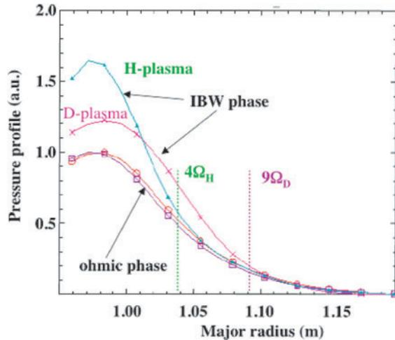
**Figure 2.** Pressure profile before (Ohmic phase) and after IBW injection in D and H discharges at 0.4 MA/7.9 T. The location of the absorption radius is also shown.
