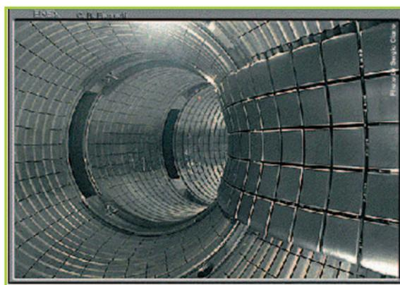
Figure 1 An internal view of the Frascati Tokamak Upgrade vessel. The limiter is shown in the central part of the chamber.
