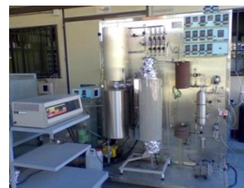
Pilot membrane gas separation plant
